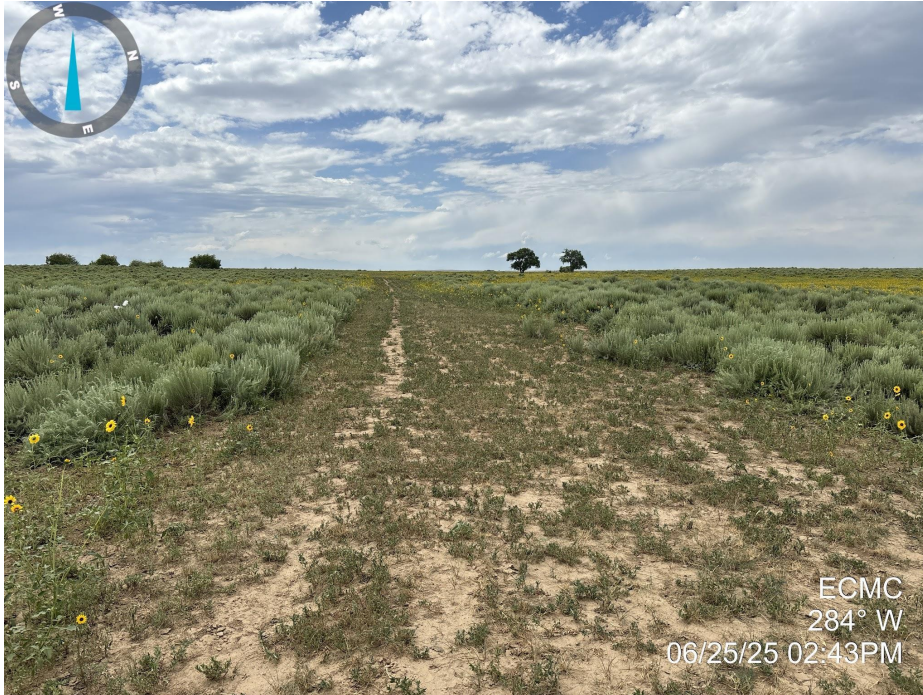
Photo 7. Photo taken of the access road to the tank battery location, facing west. Photo illustrates that final reclamation activities have taken place, with evidence of drill row seeding, but vegetation has not established to Rule 1004 standards.
