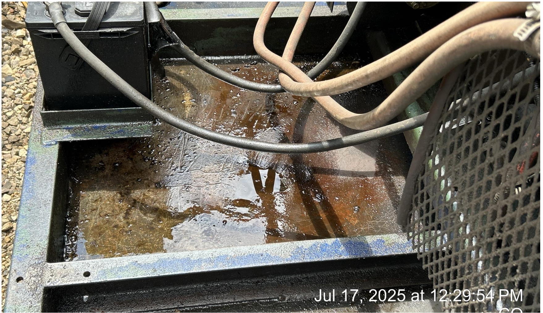
PHOTO 5: OIL IN SKID ENGINE
