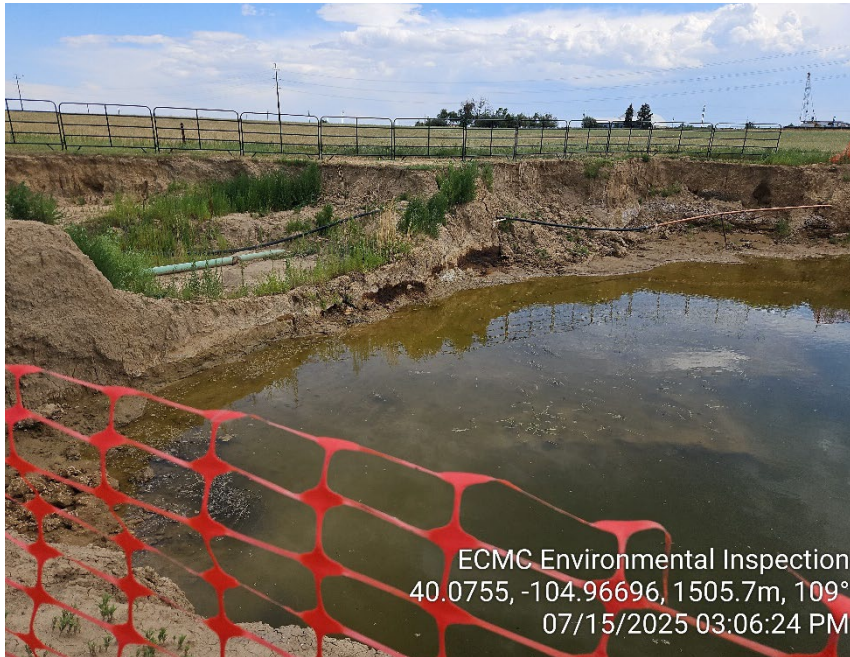
Photo 5 – Impacts visible within open excavation. Free product was observed pooling on soil next to groundwater. Weeds.
