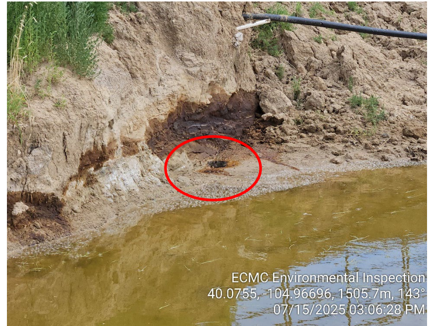
Photo 6 - Impacts and free product in open excavation.
