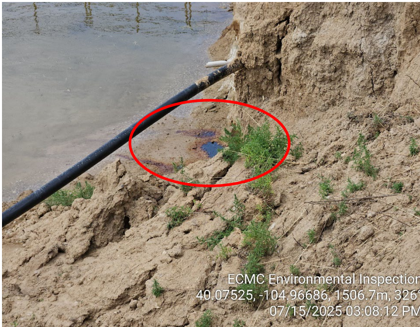
Photo 7 – Impacts and free product in open excavation. Sheen visible on groundwater.
