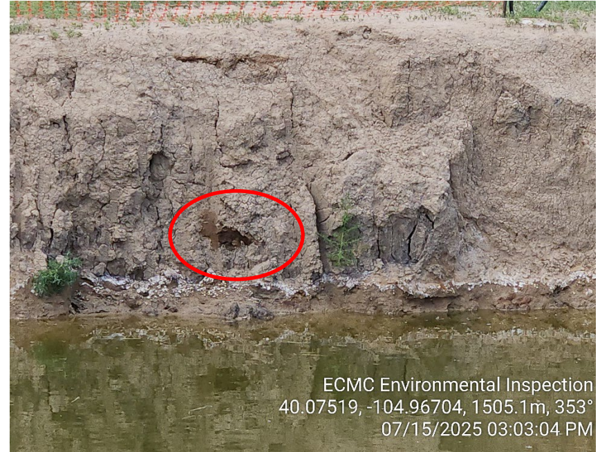
Photo 4 - Hydrocarbon impacts visible on north excavation sidewall.
