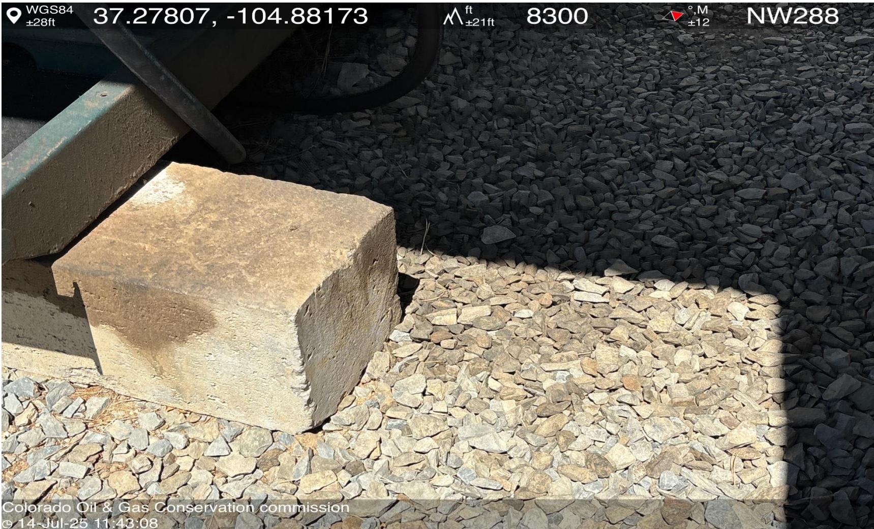
PHOTO 8: AREA OF IMPACTED SOIL PRIME MOVER ENGINE SKID. Conduct maintenance on equipment, cleanup stained material and review self inspection processes. COMPLY WITH RULE 1002,.(2).D. CA DATE 7-25-2025.
