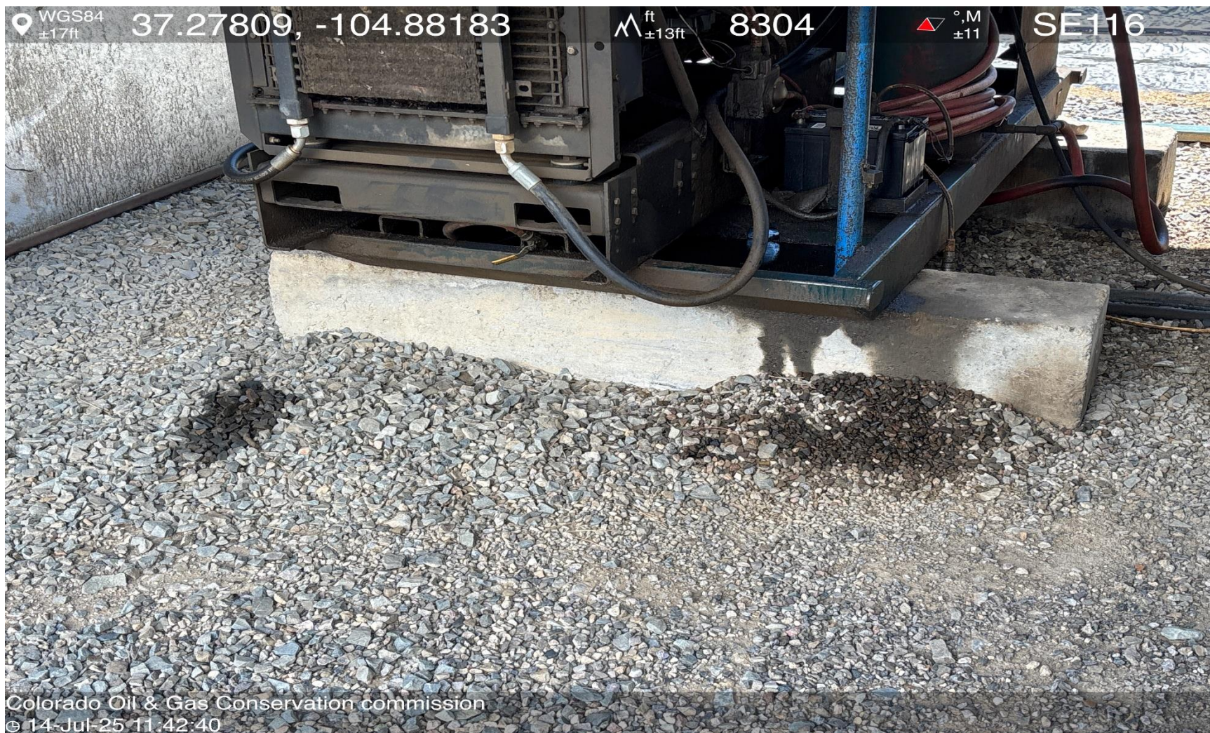
PHOTO 7: AREA OF IMPACTED SOIL PRIME MOVER ENGINE SKID. Conduct maintenance on equipment, cleanup stained material and review self inspection processes. COMPLY WITH RULE 1002,(2).D. CA DATE 7-25-2025.
