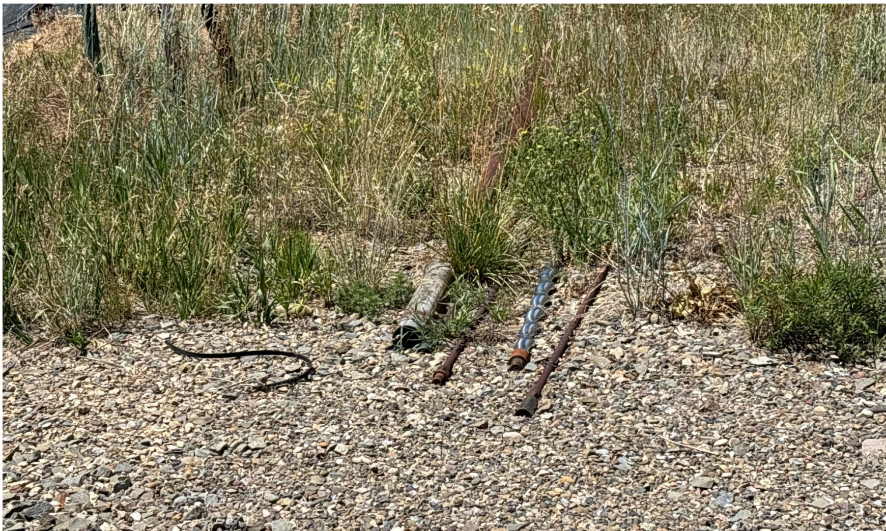
PHOTO 5: UNUSED EQUIPMENT STORED ON LOCATION (PUMP, POLISH ROD AND RODS). REMOVE UNUSED EQUIPMENT PER RULE 606. CA DATE 7-25-2025.
