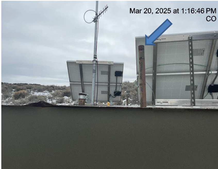
Photo # 5853 From inspection 708906068 conducted on 03/20/2025 PRV vent line does not comply with CECMC pressure safety device rules
