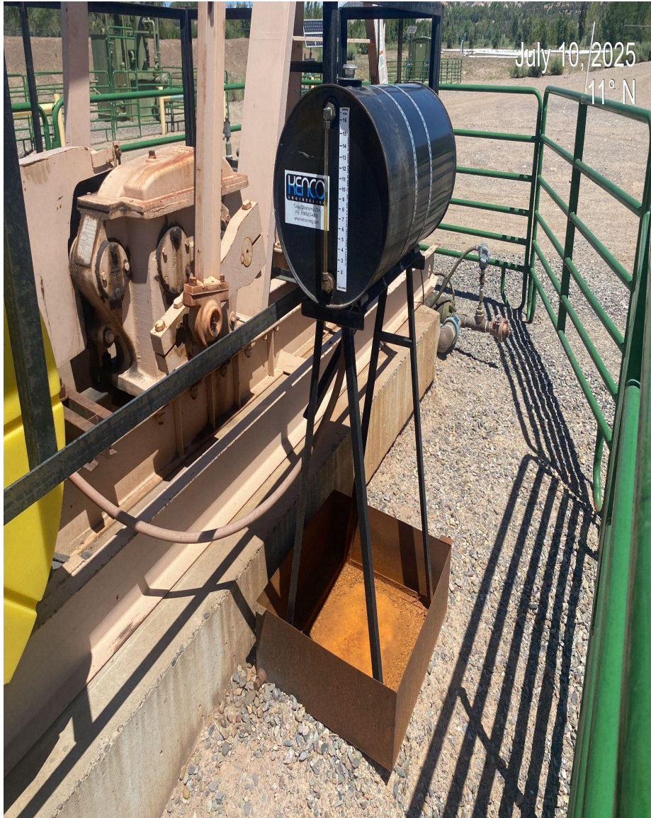
Photo 3. Lube tank secondary containments at both pump jacks have no wildlife cover/protections.
