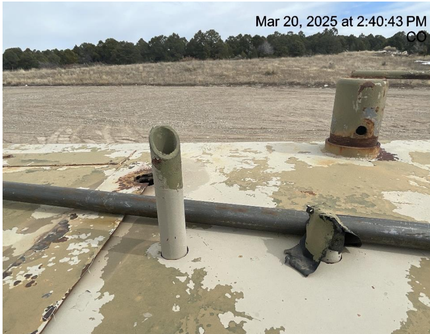
Photo # 6183 From inspection/audit 708906074 conducted on 03/20/2025 PRV vent line on separator does not comply with CECMC pressure safety device rules
