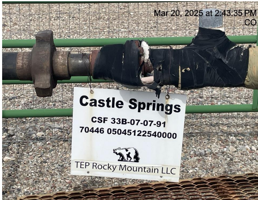
Photo # 6185 From inspection/audit 708906074 conducted on 03/20/2025 Wellhead sign lacks required information
