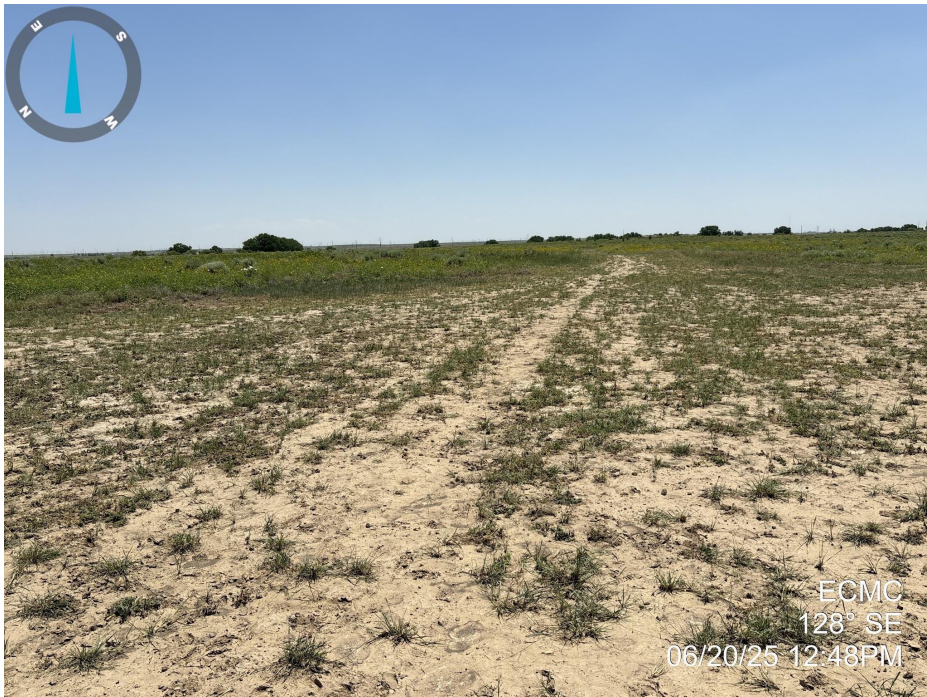
Photo 5. Photo taken of the access road to the well location, facing Southeast. Photo illustrates that final reclamation activities have taken place, with evidence of drill row seeding, but vegetation establishment does not meet Rule 1004 standards.
