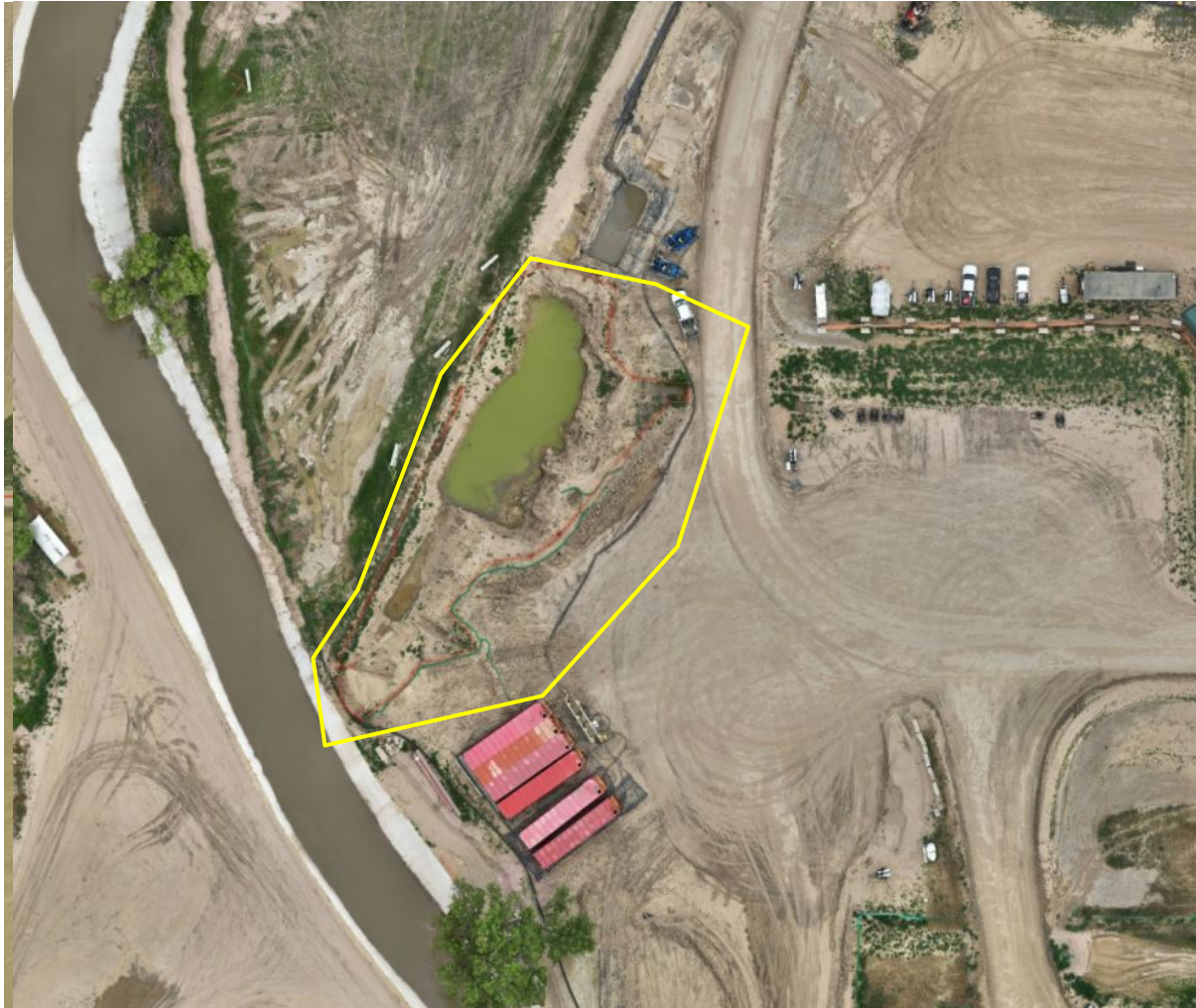
Photo 5. ECMC drone aerial imagery illustrates the emergency pit areas (yellow area). The southern emergency pit area has insufficient BMPs around unconsolidated bermed material. See Photo 6.
