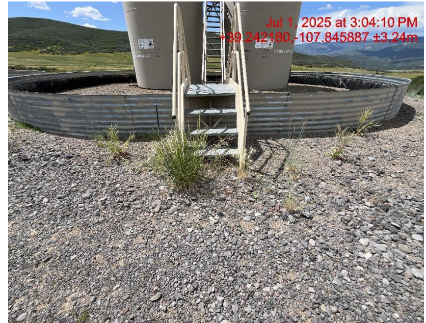
Photo # 9396 Weeds/undesirable plant species surrounding production equipment constitutes a fire hazard
