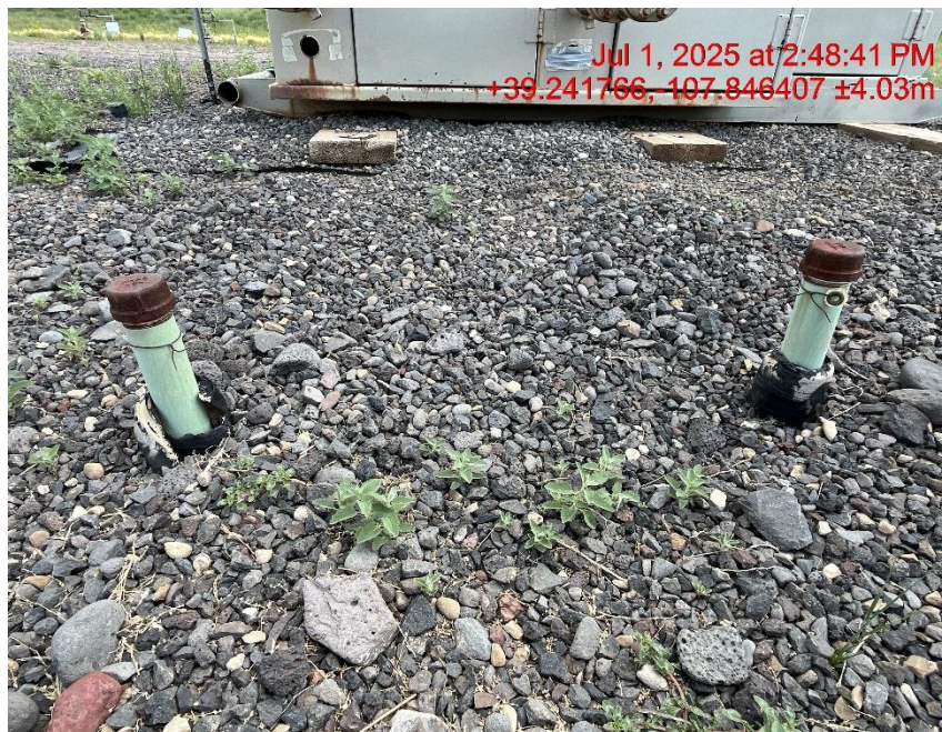
Photo # 9375 Multiple unused flowlines do not comply with CECMC 600 & 1100 series rules
