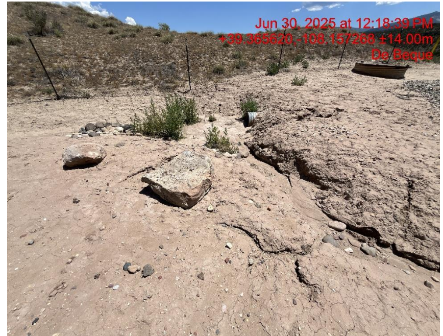
Photo # 9152 Failure to minimize erosion & transport of sediment/insufficient BMP's
