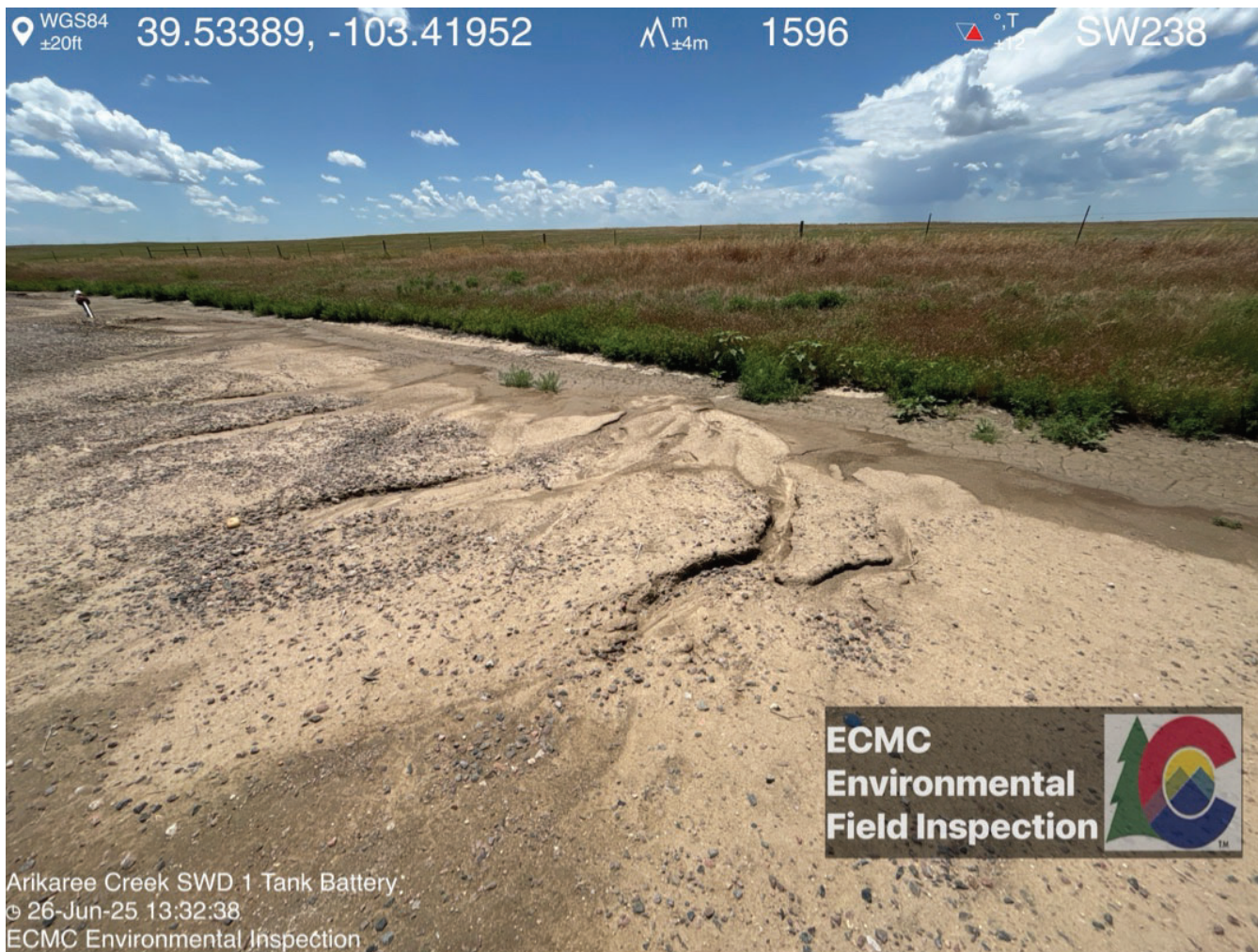
Stormwater erosion. Rill formation. Weeds.
