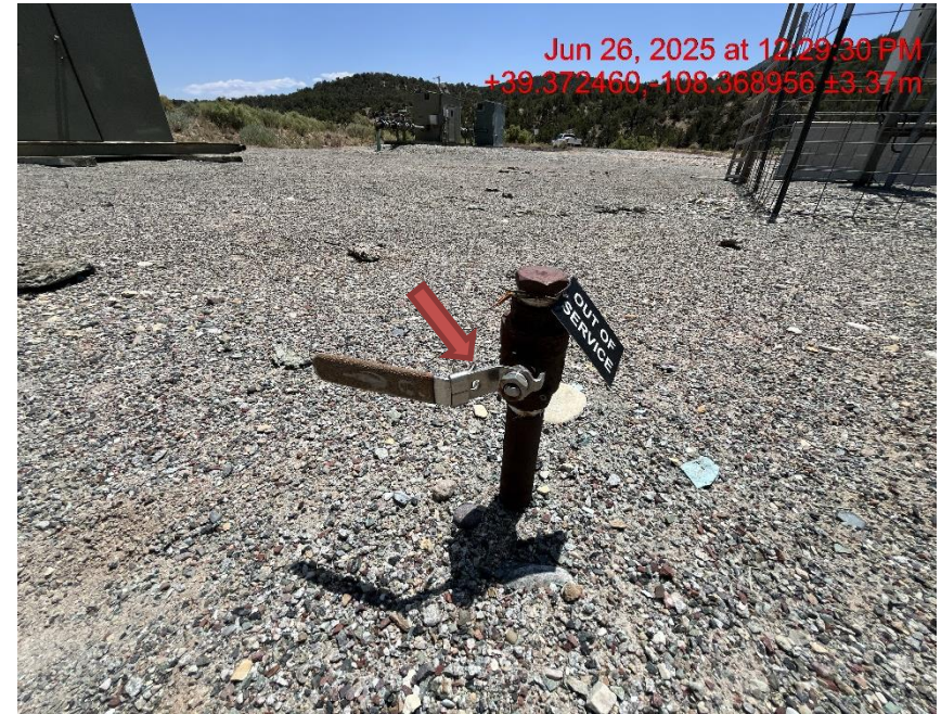
Photo # 8893 Unused flowline does not comply with CECMC 600 & 1100 series rules
