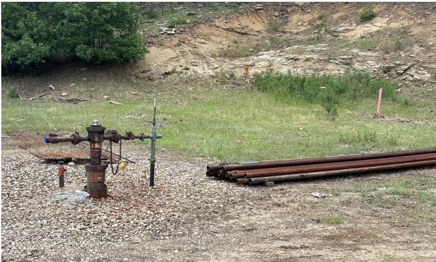
PHOTO 4: UNUSED EQUIPMENT STORED ON LOCATION (TBG & RODS). REMOVE UNUSED EQUIPMENT PER RULE 606. CA DATE 7-9-2025.
