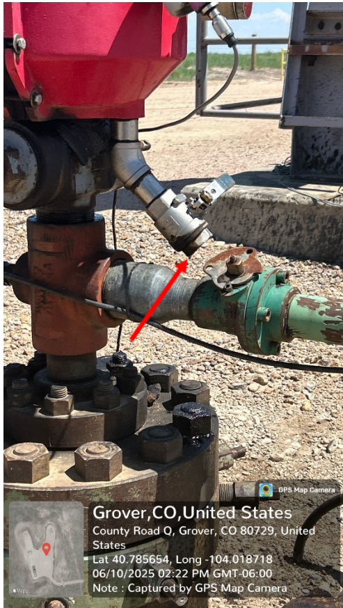
Photo 4 – Active drip from closed value and plug
