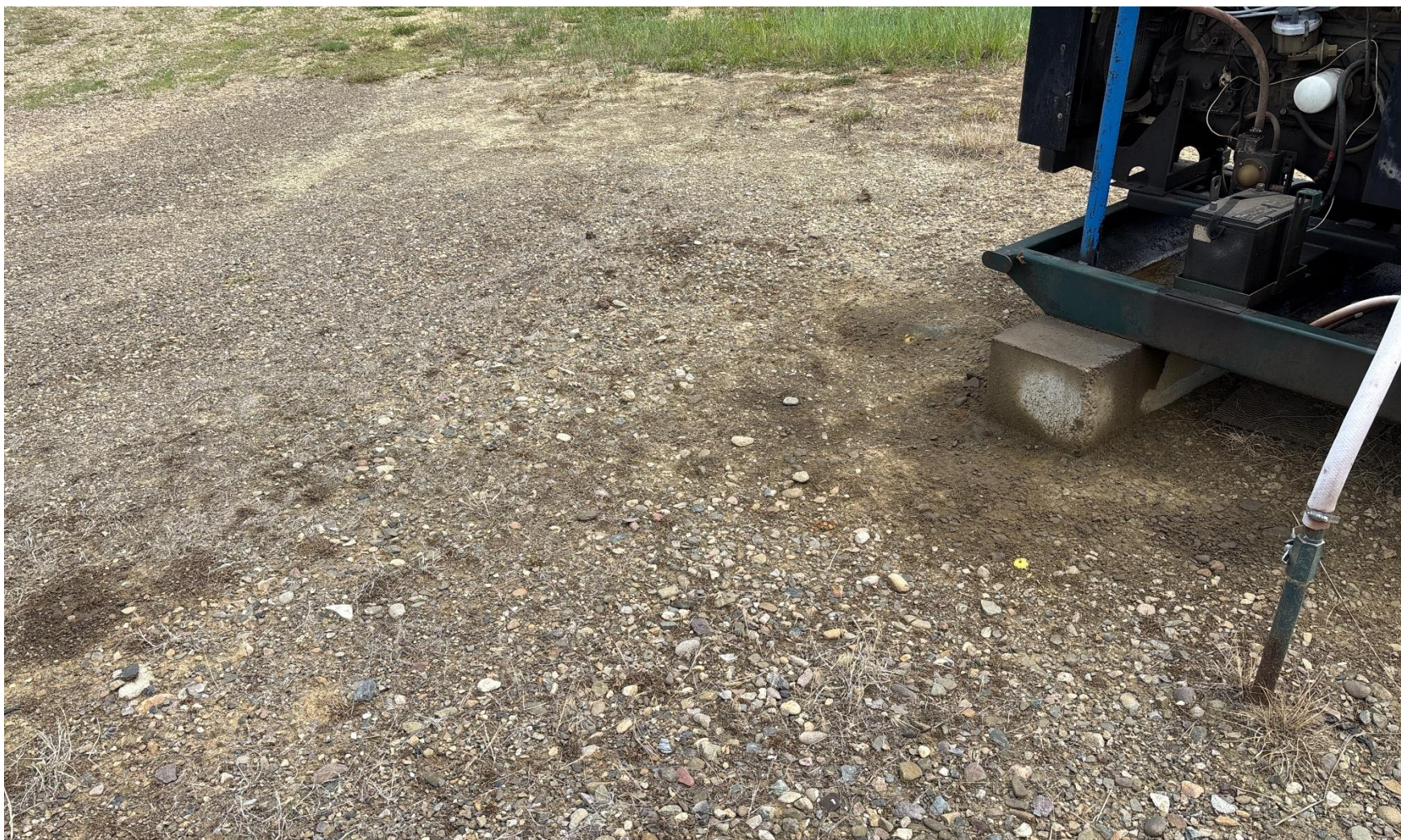
PHOTO 5: AREAS OF IMPACTED SOIL STARTING AT PRIME MOVER ENGINE SKID GOING TOWARD ORIGINAL WELLHEAD. Conduct maintenance on equipment, cleanup stained material and review self inspection processes. COMPLY WITH RULE 1002,(2).D CA DATE 6-26-2025.
