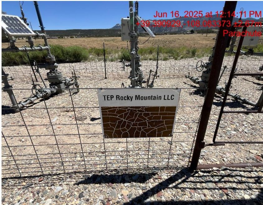
Photo # 8581 Wellhead signs are not legible
