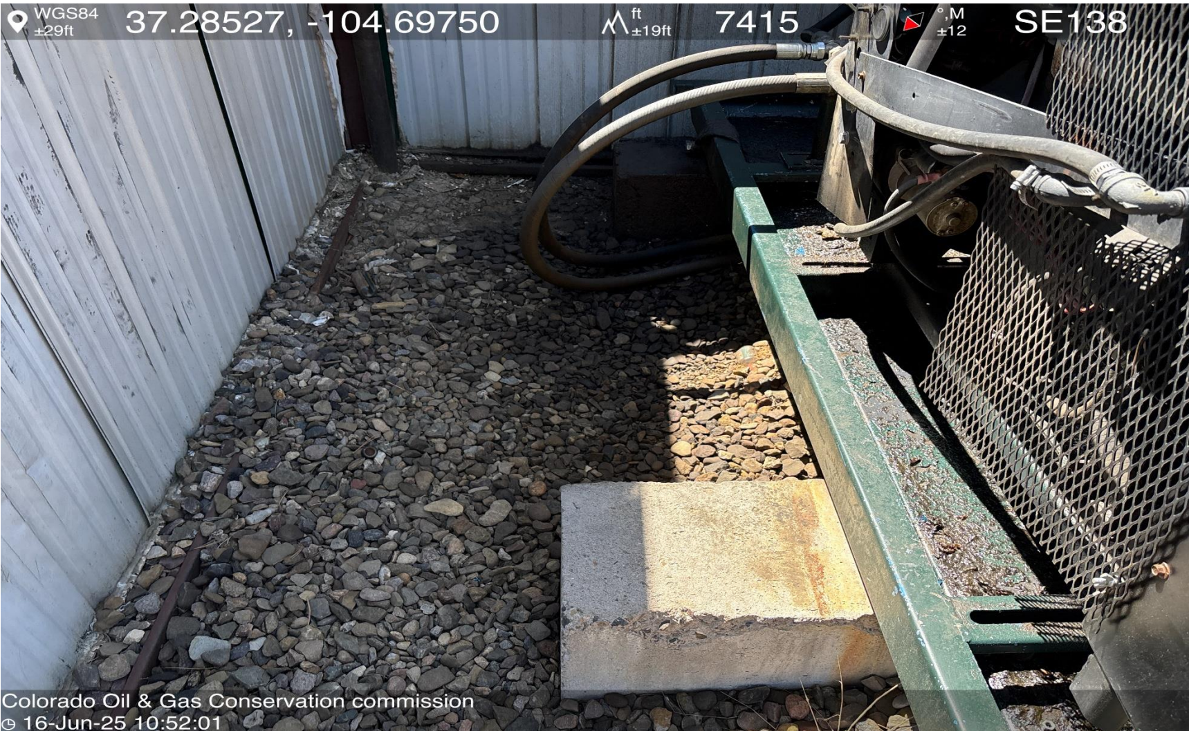
PHOTO 8: AREA OF IMPACTED SOIL AROUND PRIME MOVER ENGINE SKID (IMPACTED SOILS ON OTHER SIDES OF SKID ALSO). Conduct maintenance on equipment, cleanup stained material and review self inspection processes. COMPLY WITH RULE 1002,.(2).D. CA DATE 6-25-2025.
