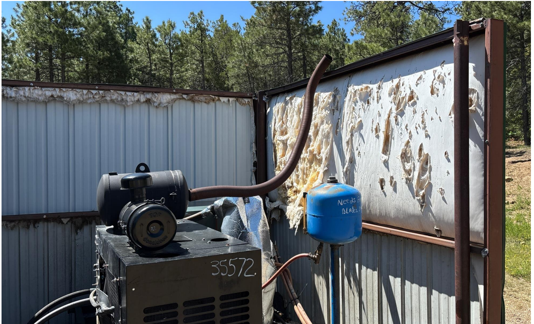
PHOTO 5: TRASH AND OR DEBREE (INSULATION ON SOUND WALLS IS DETERIORATING AND SPREADING ON AND AROUND LOCATION). PICK UP ALL TRASH ON AND AROUND LOCATION AND SECURE OR REPLACE INSULATION PER RULE 606. CA DATE 6-25-2025.
