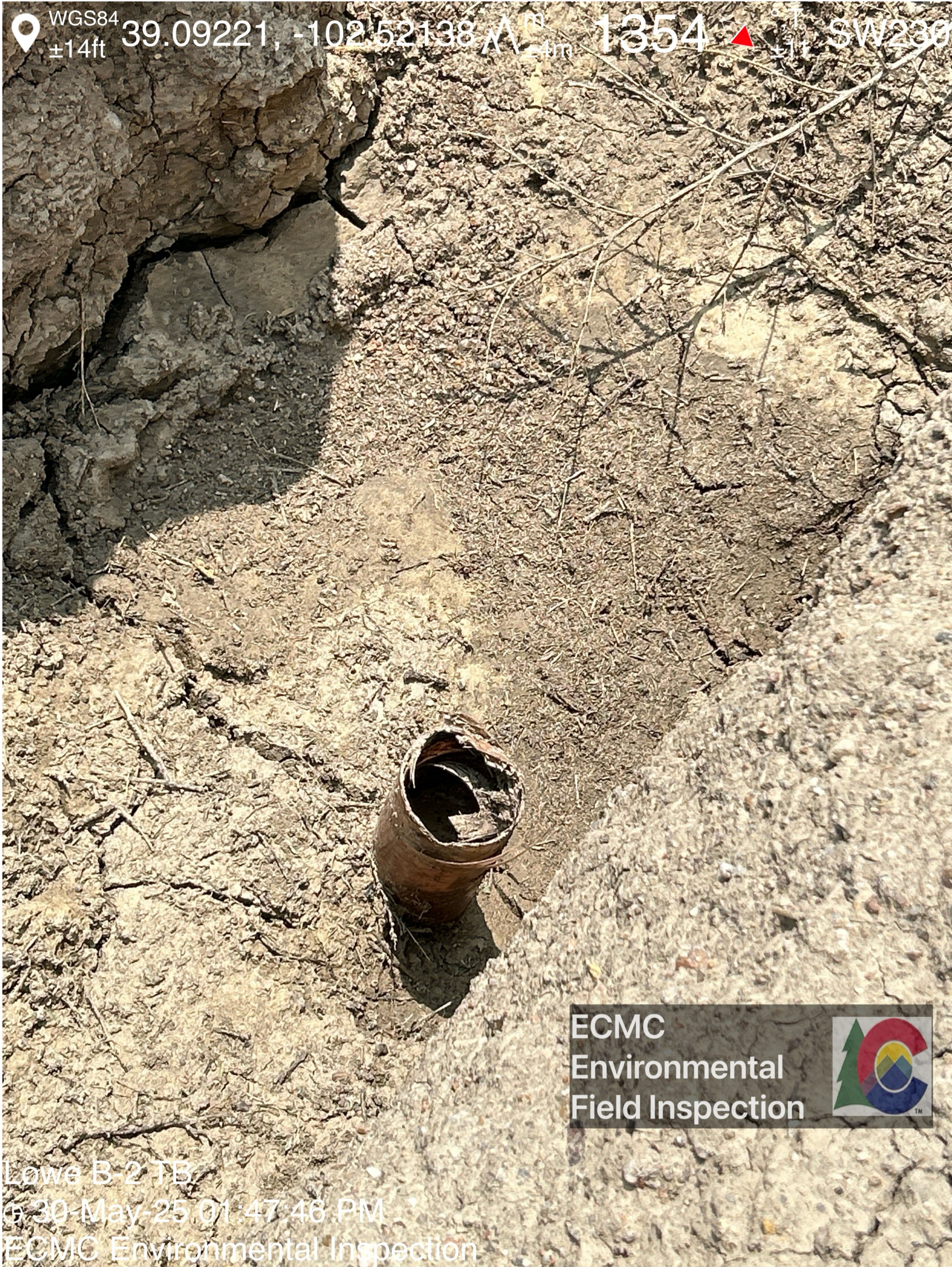
The uncapped riser appears to consist of fiberglass.
