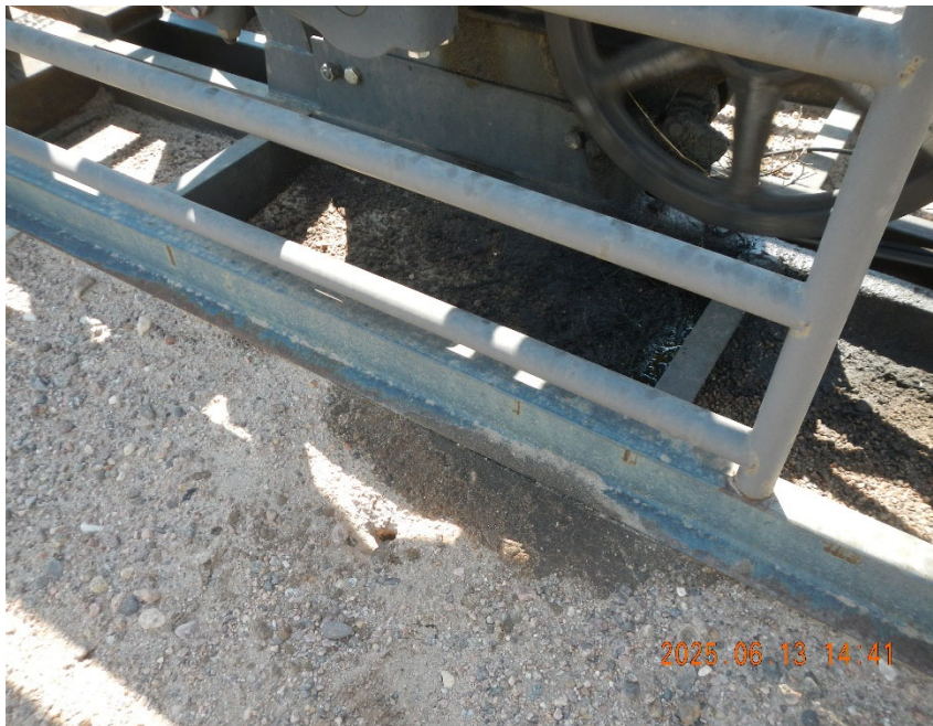
3. View of stained soil at gear box.
