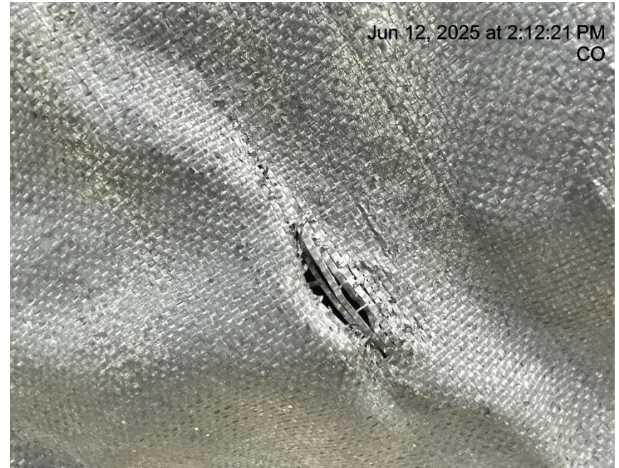
Photo # 8639 Hole in liner/liner needs maintenance
