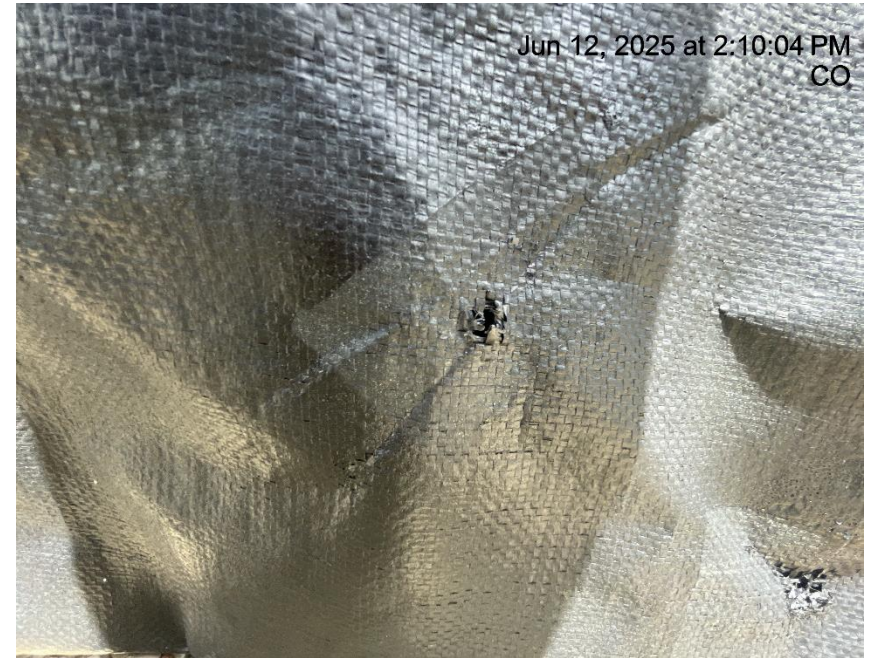
Photo # 8933 Holes in liner/liner needs maintenance
