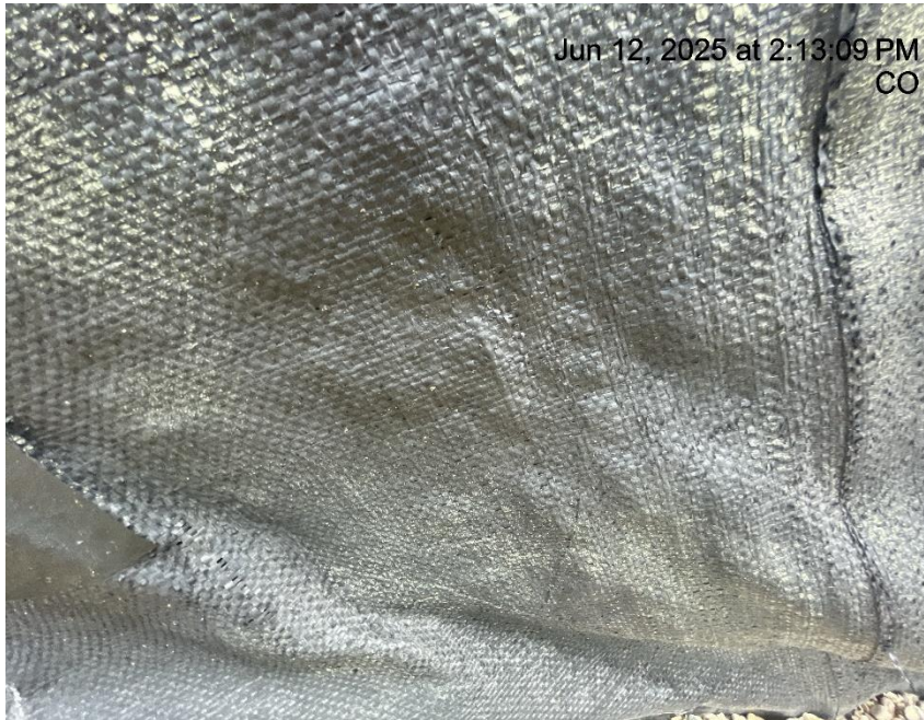
Photo # 8646 Liner deteriorating/liner needs maintenance
