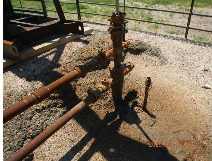
2. View of wellhead. Note ground wet around wellhead from leak at packing.
