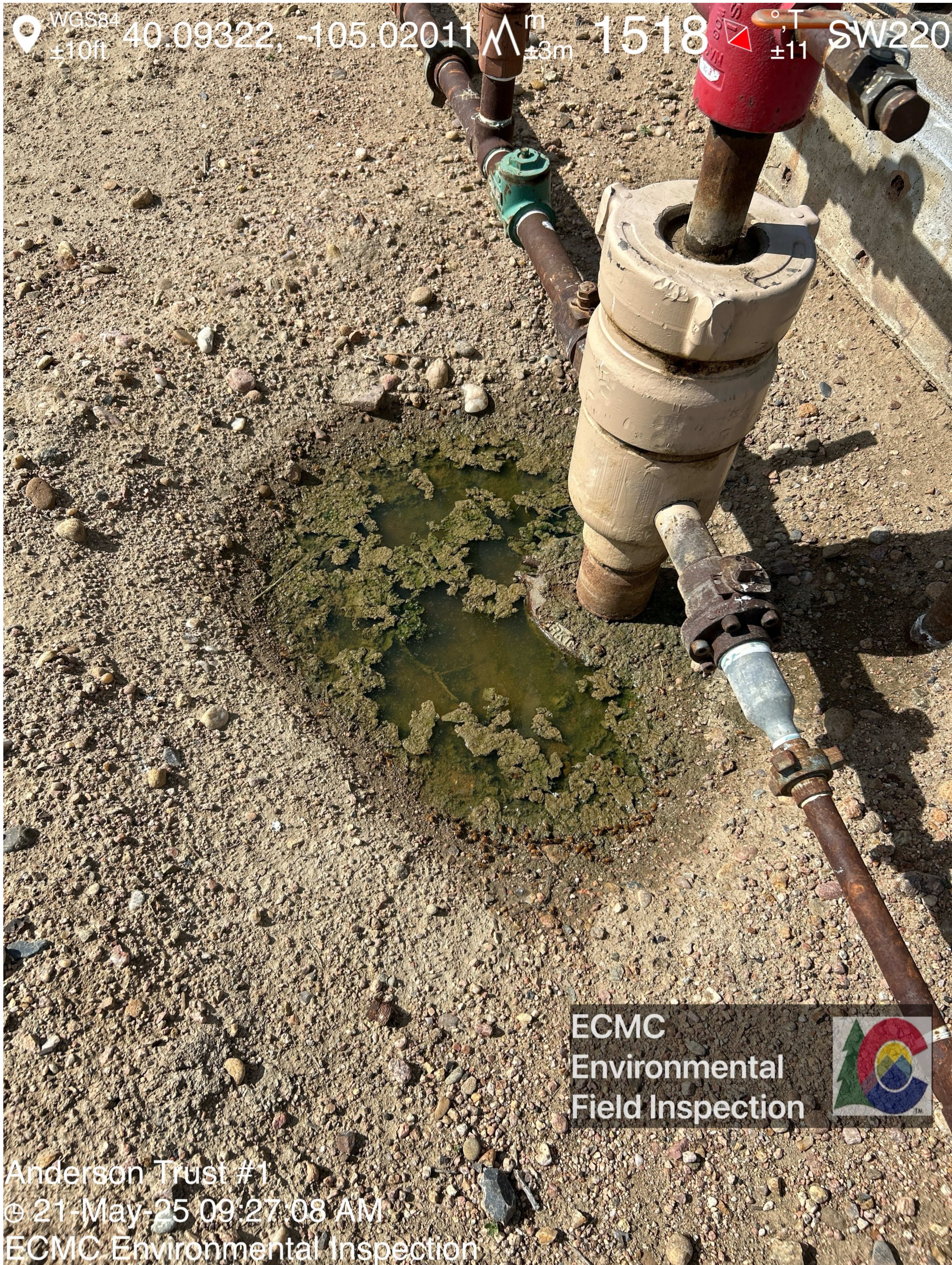
Pooled fluid is visible around the wellhead. Inspects were visible swarming the pooled fluid.
