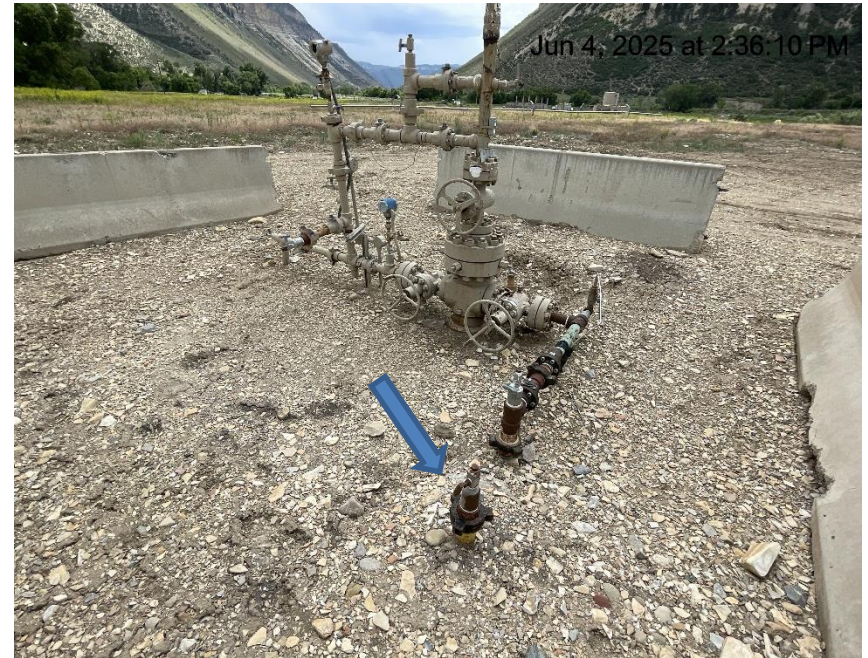
Photo # 6390 Unused flowline does not comply with CECMC rules
