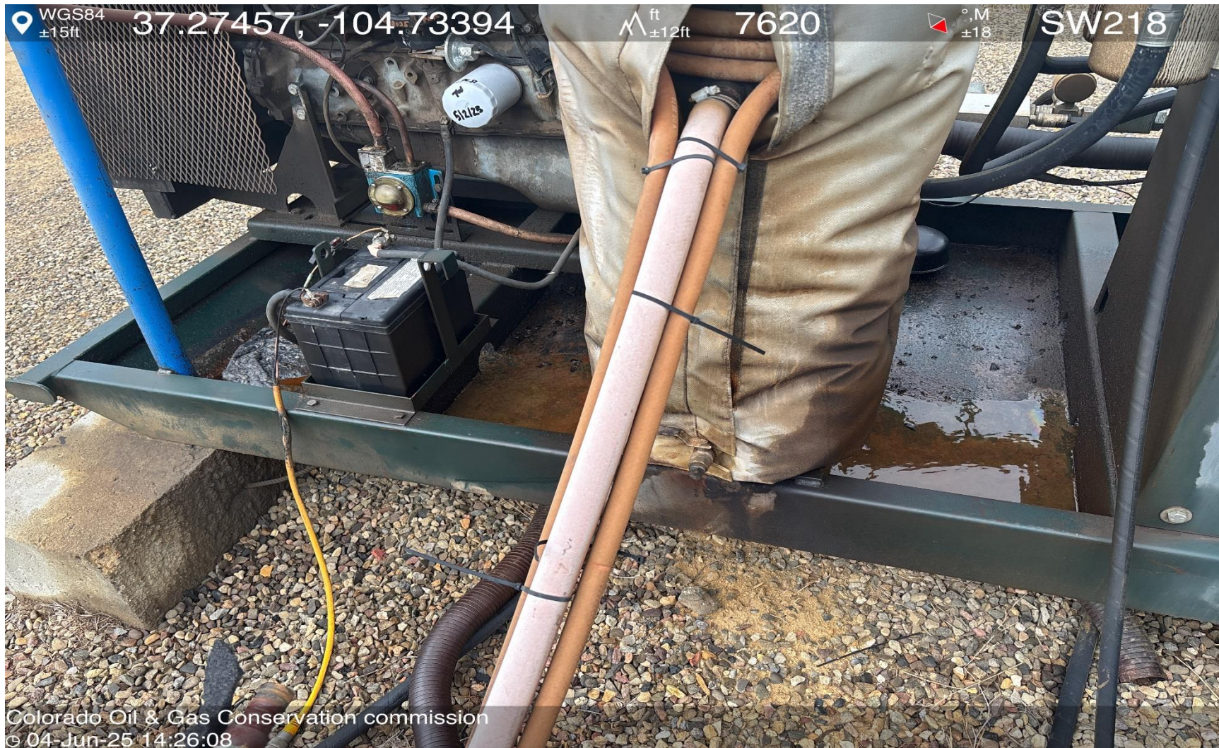
PHOTO 6: OILY WASTE IN PRIME MOVER SKID. DRAIN OILY WASTE REPAIR ALL LEAKS AND REMOVE IMPACTED SOIL PER RULE 1002..(2).D & 1002.f.(2)B, Comply with general provisions of the oil and gas act for wildlife protection AND SB-181. CA DATE 6/5/2025.
