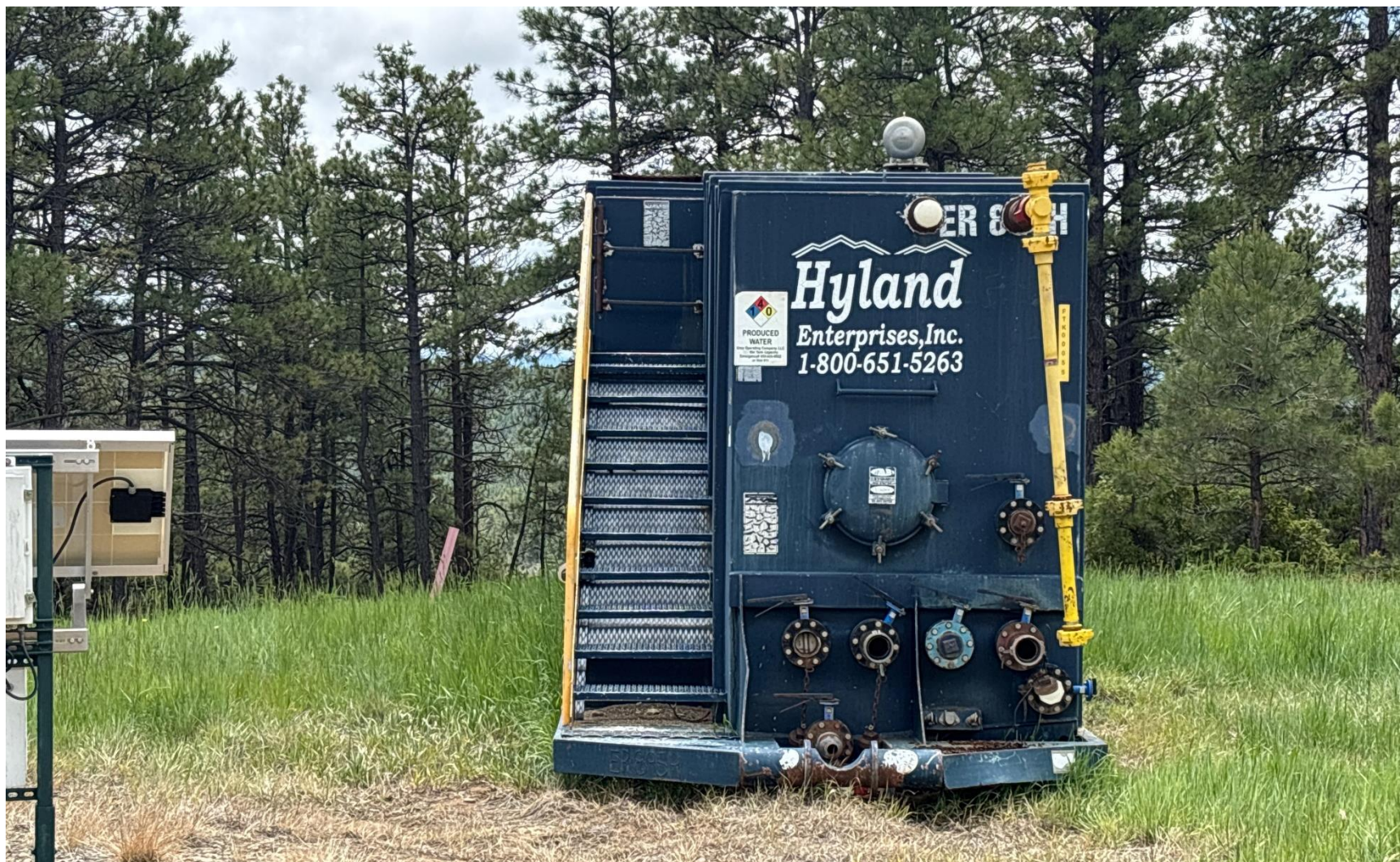
PHOTO 5: APPEARS TO BE UNUSED TANK BATTERY. IF PRODUCED WATER TANK IS NOT NECESSARY FOR THE OPERATION OF THIS WELL IT MUST BE REMOVED PER RULE 606. IF TANK IS NECESSARY FOR THE OPERATION OF THIS WELL A BERM MUST BE INSTALLED AROUND TANK PER RULE 603.o.
