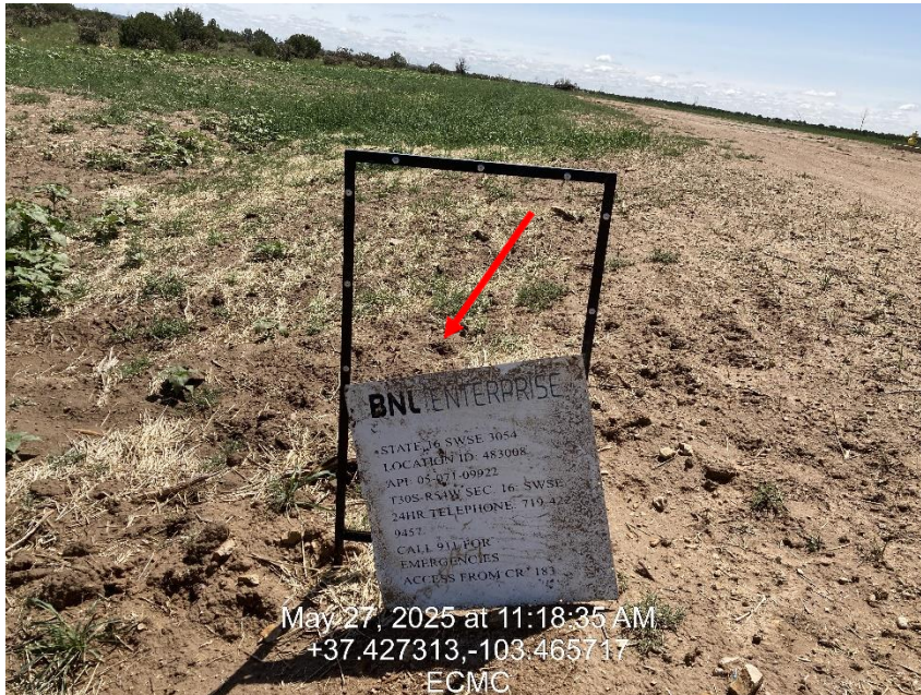
Photo 3 – Well placard has not secured to frame
