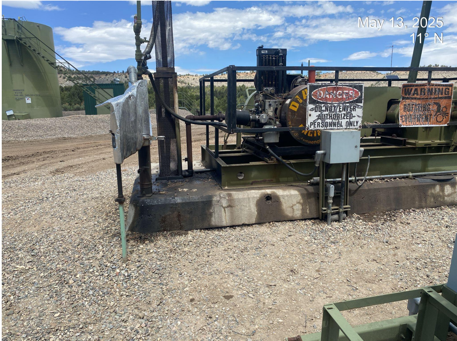
Photo 3. Spill/Stained soils observed at pumpjack equipment.
