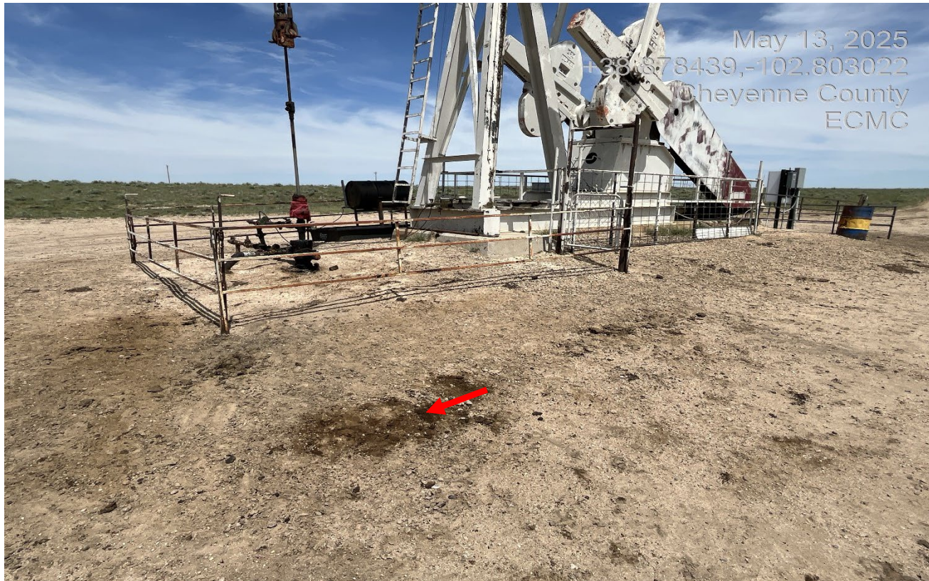
Photo 4. There are stained oily soils from a leak at the wellhead. Stained soils have not been cleaned up since the previous inspection.
