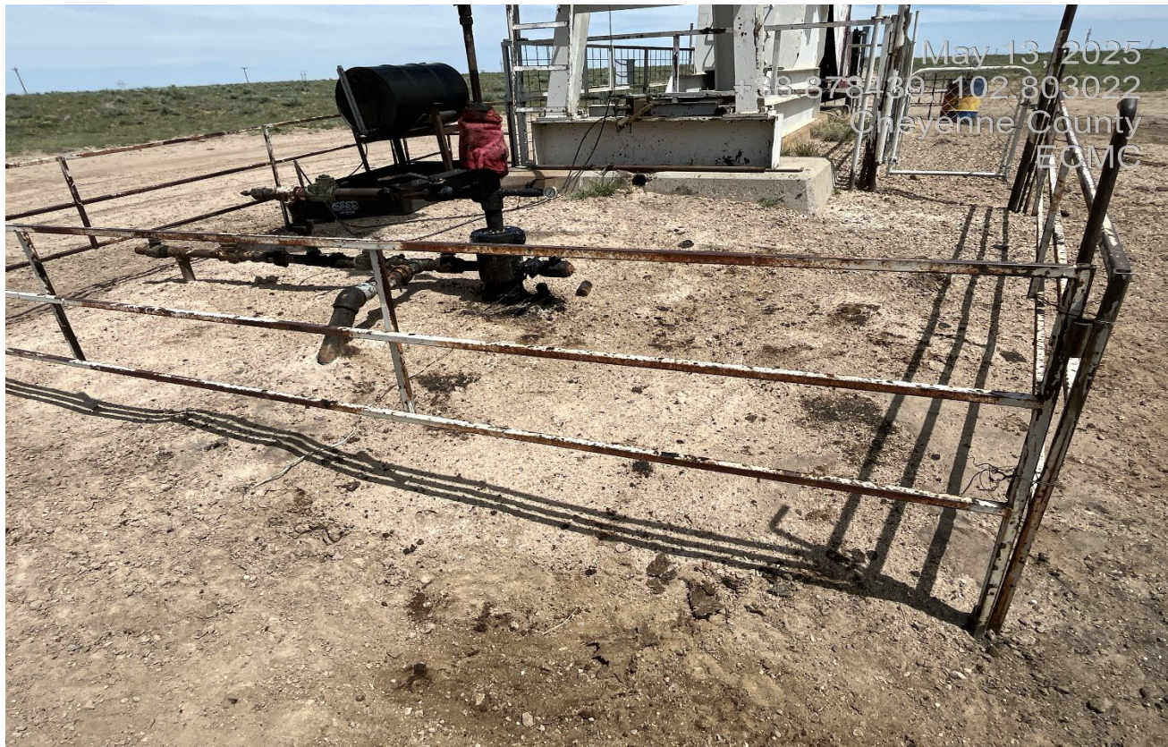
Photo 6. View of wellhead shows stained soils which were previously covered up with sand. Stained soils have not been cleaned up since the previous inspection. The well still appears to be dripping oil.
