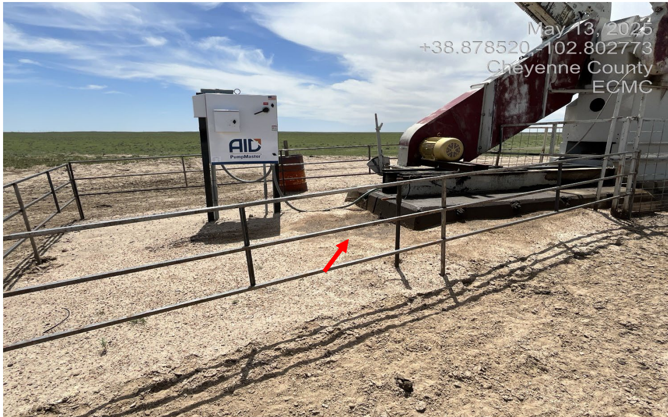
Photo 7. There are still oil stained soils at the pumpjack that have not been cleaned up. Previous corrective action was not completed.
