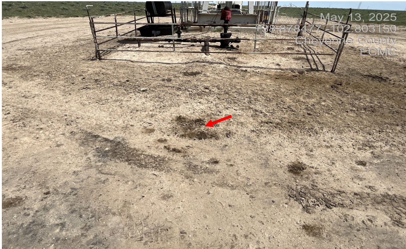
Photo 5. Facing east toward the wellhead. There are still oil stained soils which have not been cleaned up since the previous inspection.
