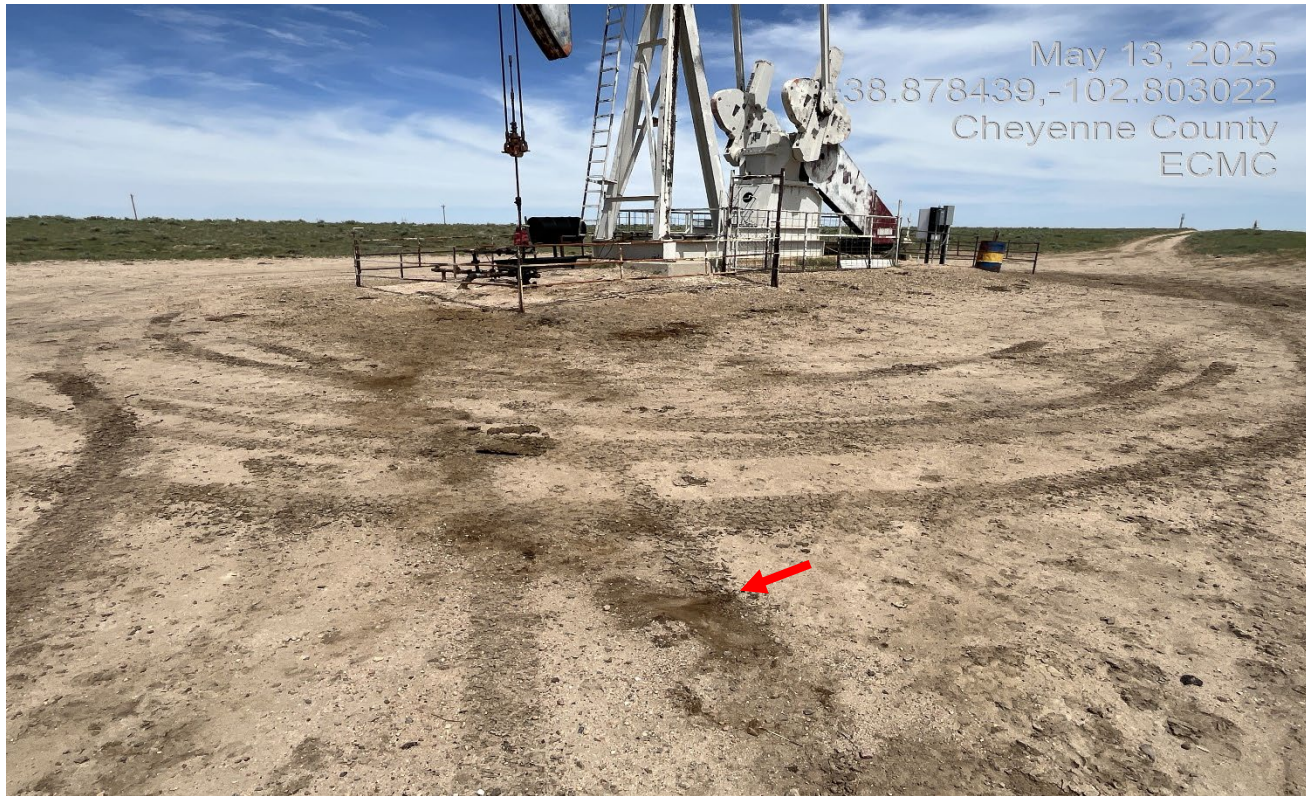
Photo 3. Facing northeast toward the wellsite. There are oil stained soils near the wellhead that have not been cleaned up since the previous inspection. The previous leak observed had flowed approximately 50 ft. to the southwest of the wellhead.
