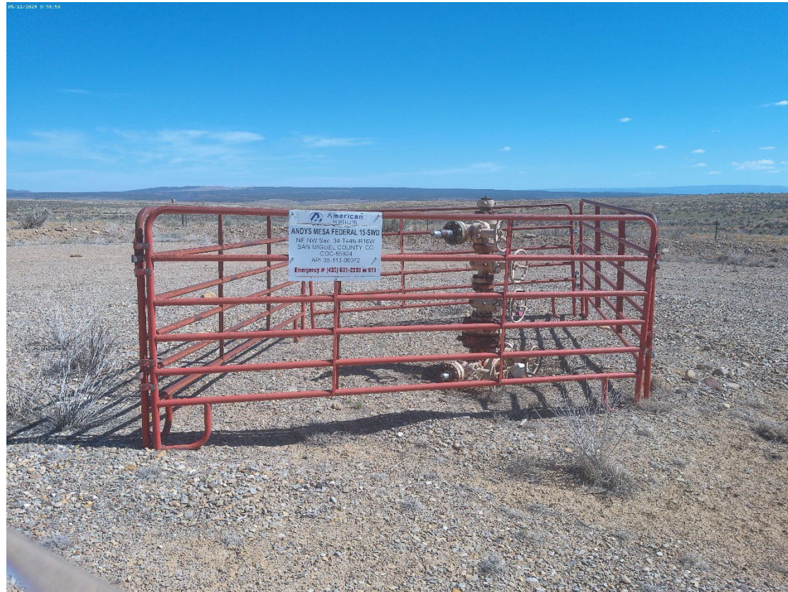
Injection Wellhead with fence
