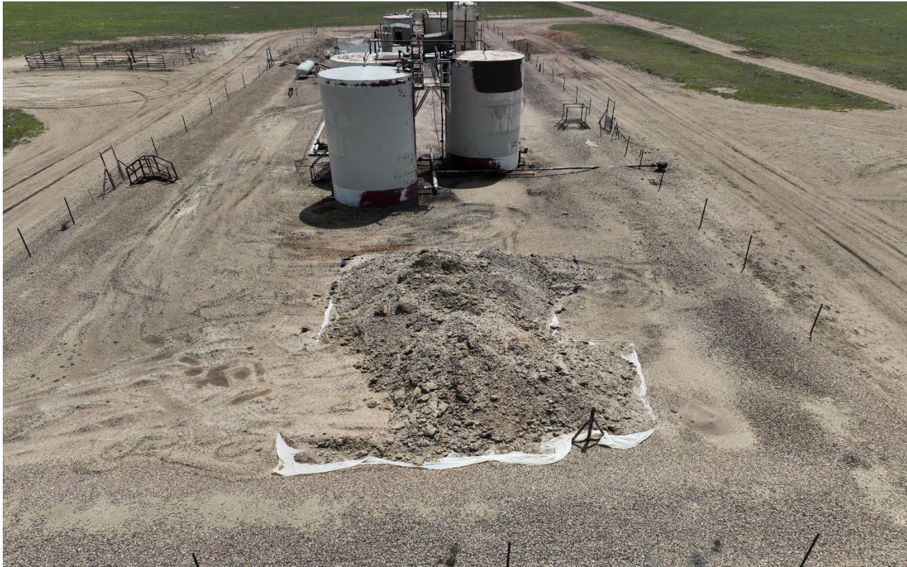
Photo 6. Drone aerial photo facing south toward the tank battery facility. E&P waste material remains on plastic liner at this area.
