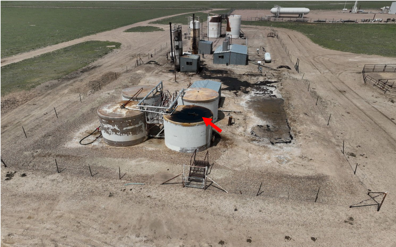
Photo 1. Drone aerial photo facing northeast toward the tank battery facility. There is a new spill that has recently occurred in addition to previous spills. The top of the tank shown at red arrow still has oily fluids that have not been cleaned up.
