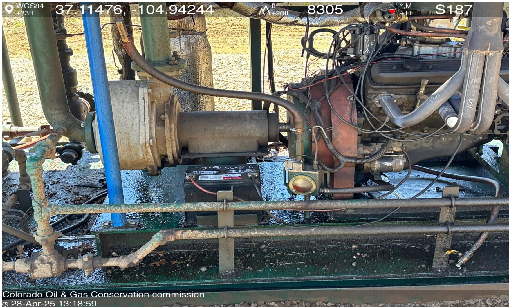
PHOTO 8: THE ENTIRE COMPRESSOR SKID IS SATURATED WITH OILY WASTE FROM SEVERE OIL LEAKS. REPAIR AND CLEAN UP EQUIPMENT.
