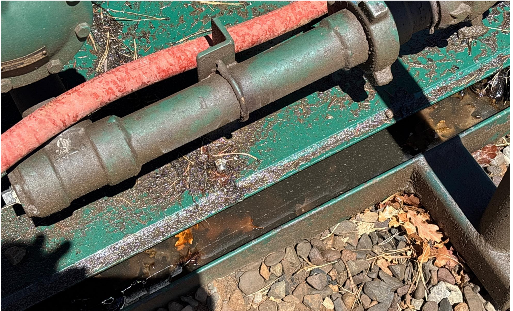
PHOTO 7: OILY WASTE IN COMPRESSOR SKID HAS NO NETTING FOR WILDLIFE PROTECTION. DRAIN OILY WASTE REPAIR ALL LEAKS AND REMOVE IMPACTED SOIL PER RULE 1002..(2).D & 1002.f.(2)B, Comply with general provisions of the oil and gas act for wildlife protection AND SB-181. . CA DATE 4-30-2025.
