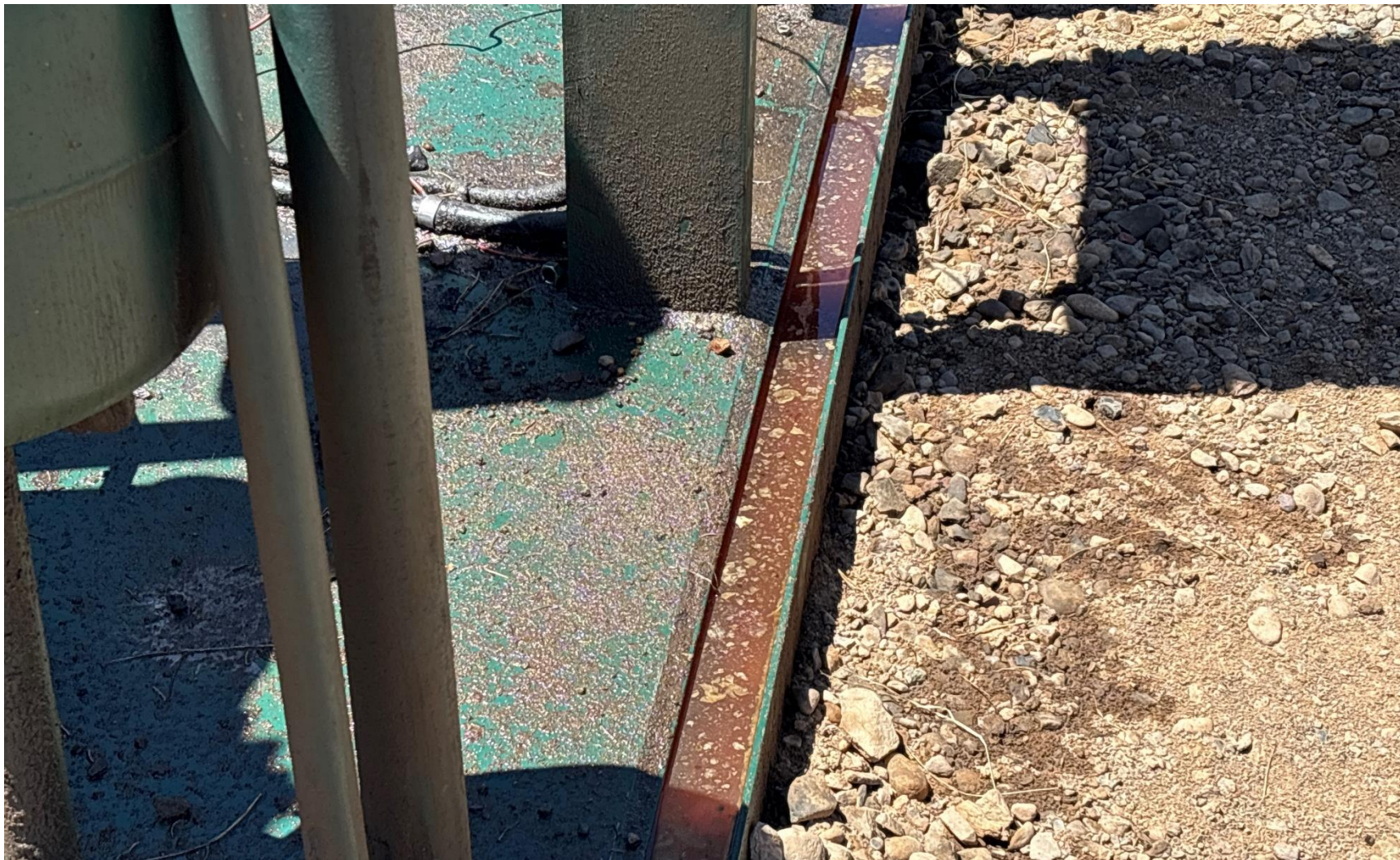
PHOTO 7: AREA OF IMPACTED SOIL NEAR COMPRESSOR. Conduct maintenance on equipment, cleanup stained material and review self inspection processes. COMPLY WITH RULE 1002,.(2).D. CA DATE 5-9-2025.
