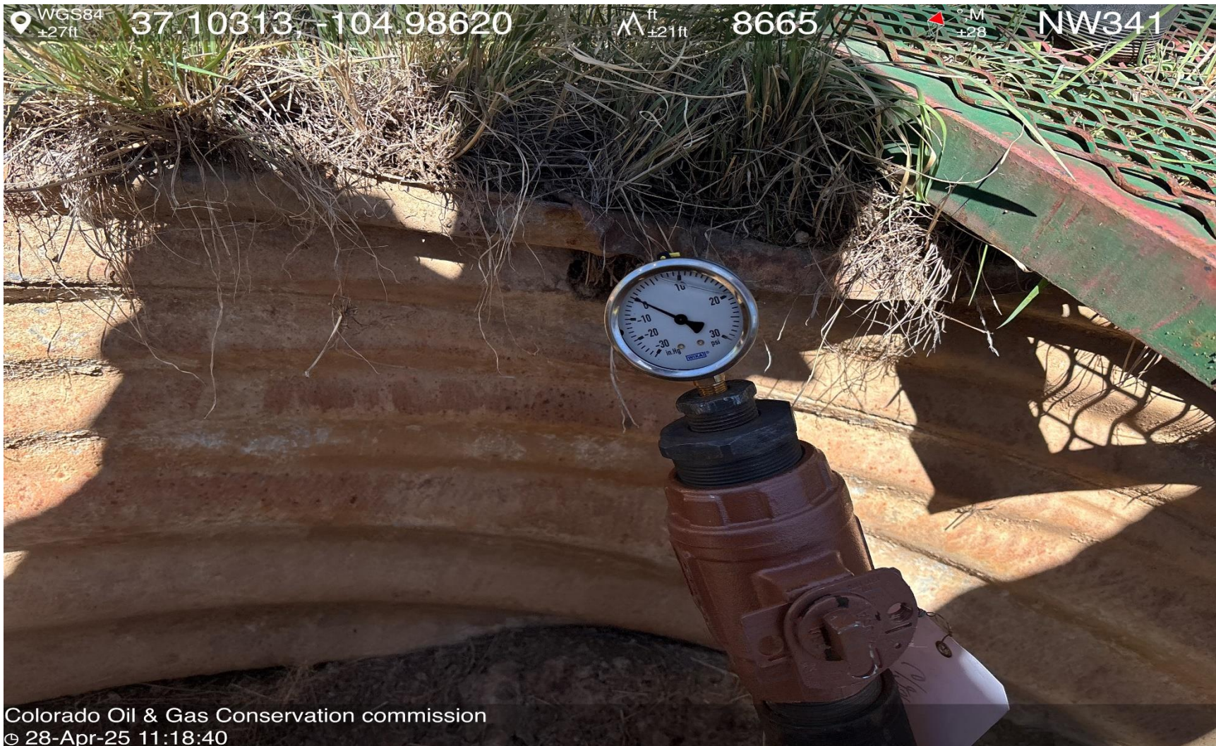
PHOTO 8: BRHD PSI 0, MONITORED OPEN FOR 15 MIN. NO BLOW NO FLOW.
