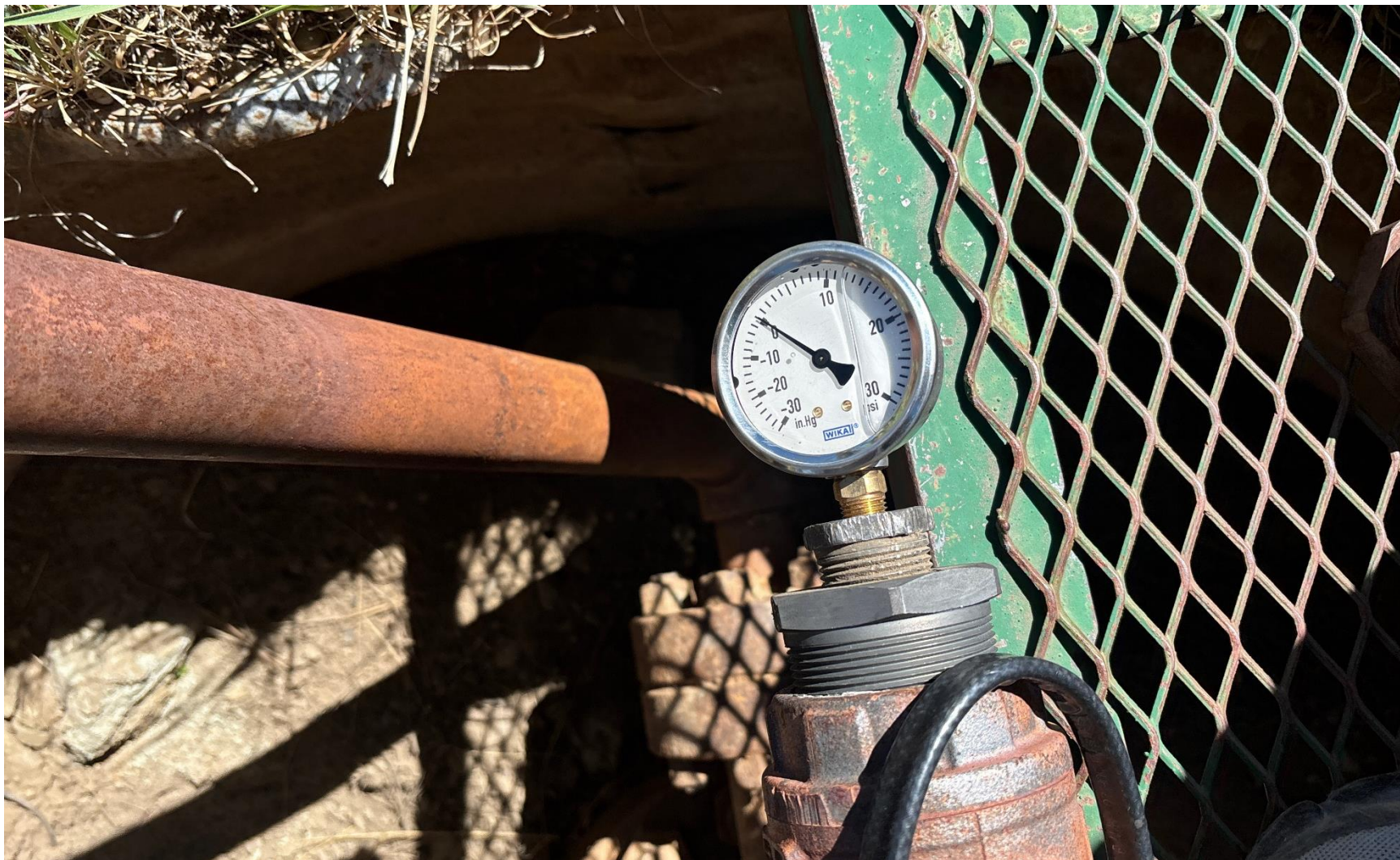
PHOTO 7: TBG PSI 0, MONITORED OPEN FOR 15 MIN. NO BLOW NO FLOW.
