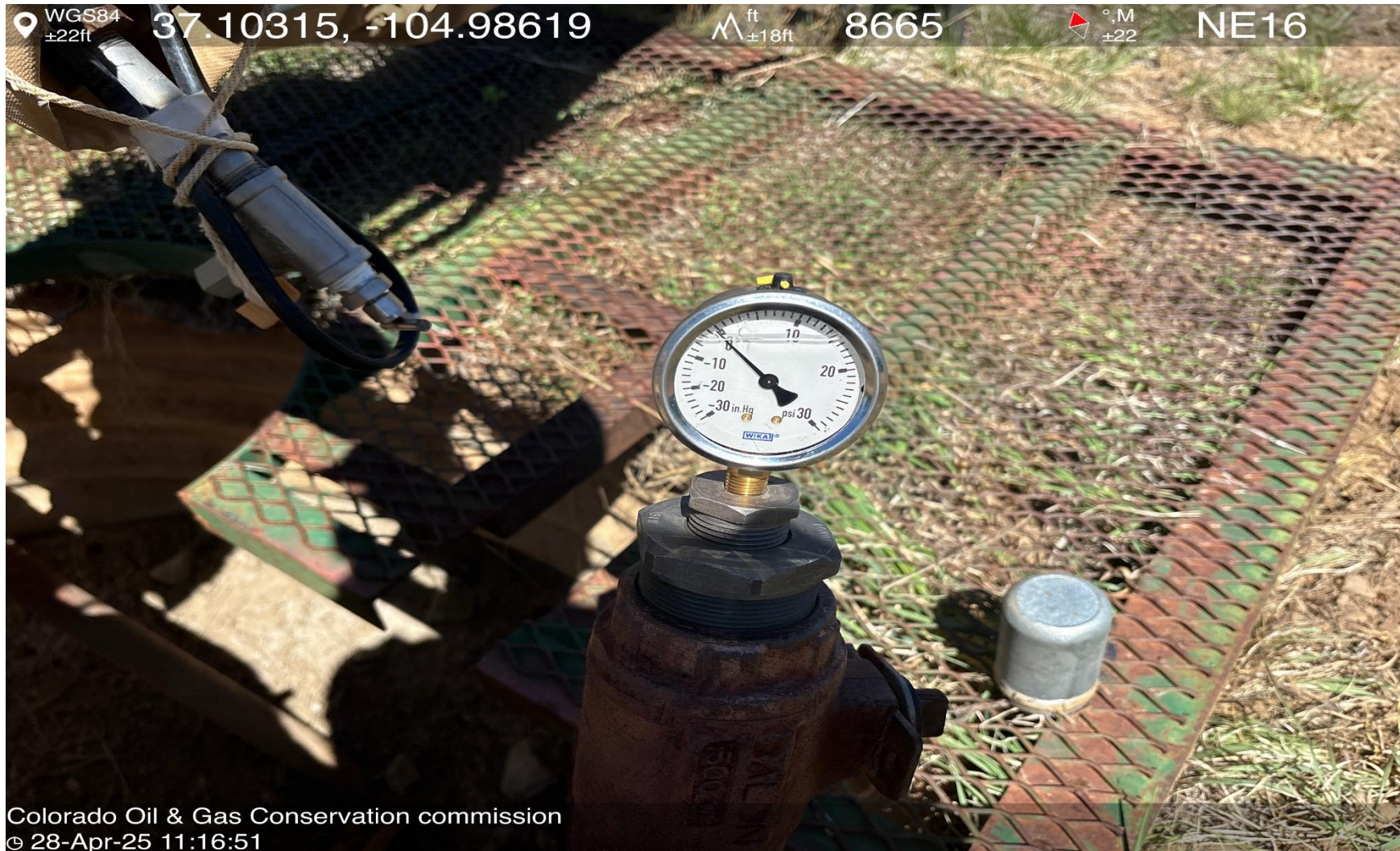
PHOTO 9: INTERMEDIATE CSG PSI 0, MONITORED OPEN FOR 15 MIN. NO BLOW NO FLOW.
