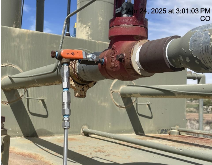
Photo # 6130 BOULTON 33-6 BH line tied into separator at the A valve bypass
