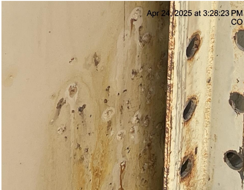
Photo # 6256 Possible tank failure - Suspected leak on production tank/tank appears to lack integrity
