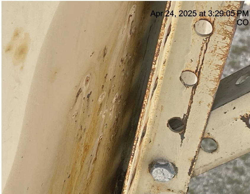
Photo # 6260 Possible tank failure - Suspected leak on production tank/tank appears to lack integrity
