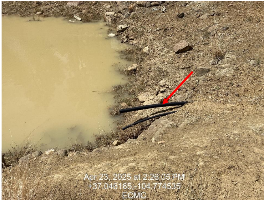
Photo 5 – Dump lines to pit.
