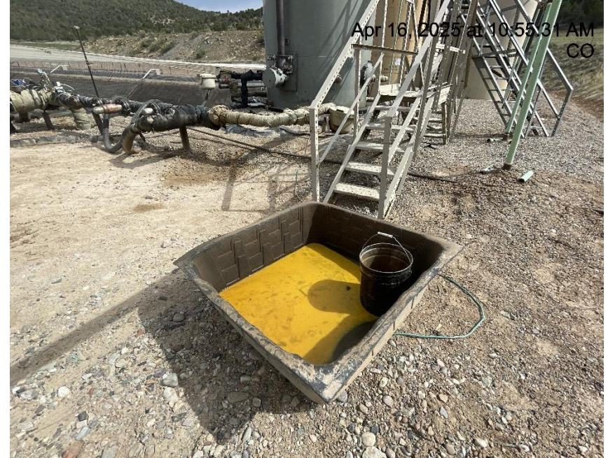
Photo # 1482 E & P waste in plastic tub/wildlife hazard & not in compliance with CECMC environmental rules
