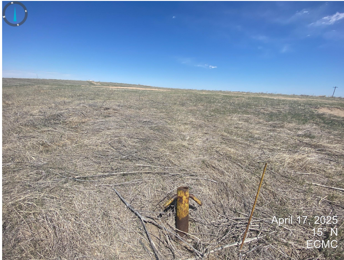
Photos 13. Guyline anchor does not appear to have been removed.
