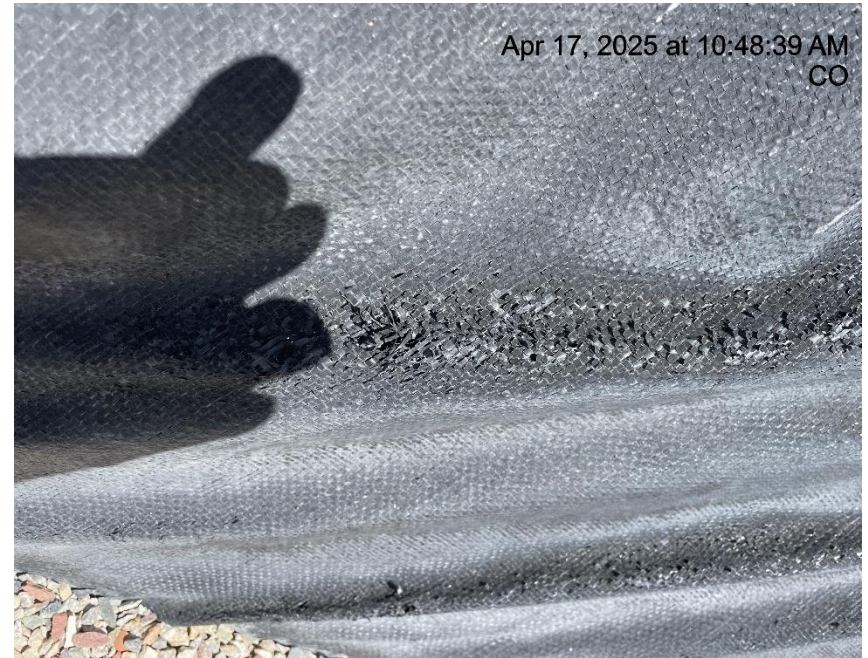
Photo # 2387 Hole in liner/liner needs maintenance & liner showing signs of deterioration
