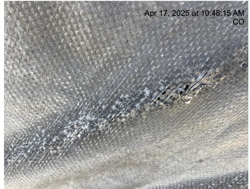
Photo # 2389 Hole in liner/liner needs maintenance & liner showing signs of deterioration
