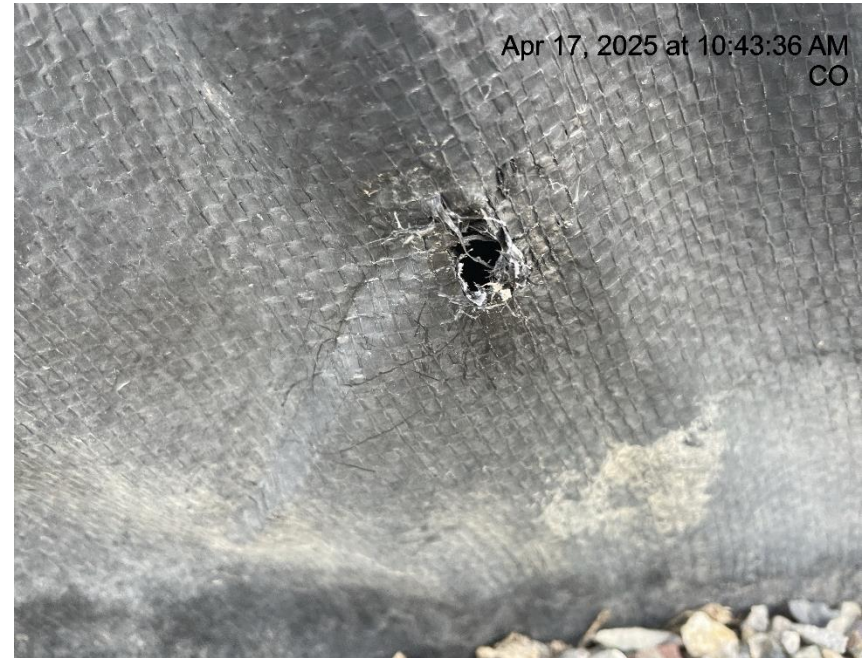
Photo # 2377 Hole in liner/liner needs maintenance
