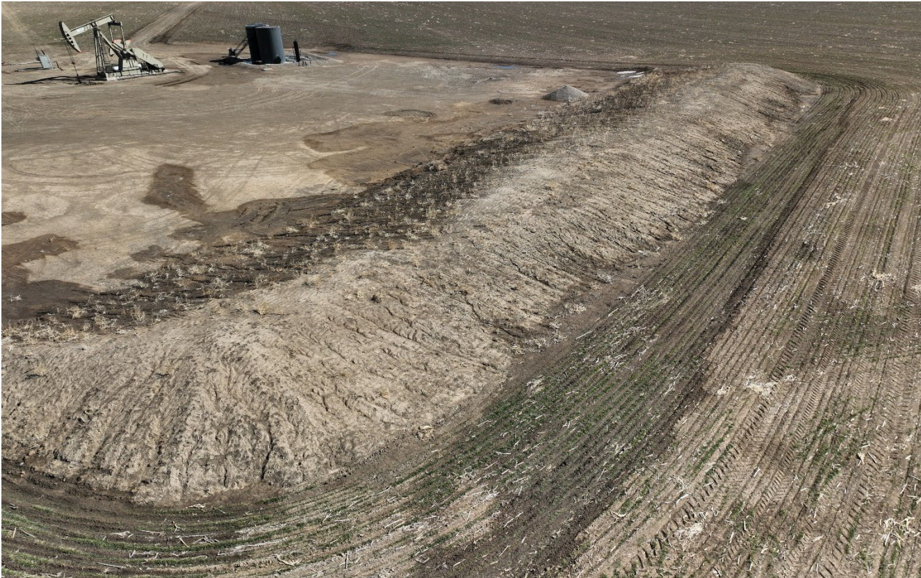
Photo 11. Drone aerial photo facing southeast toward the topsoil pile. There is erosion occurring along the topsoil pile.
