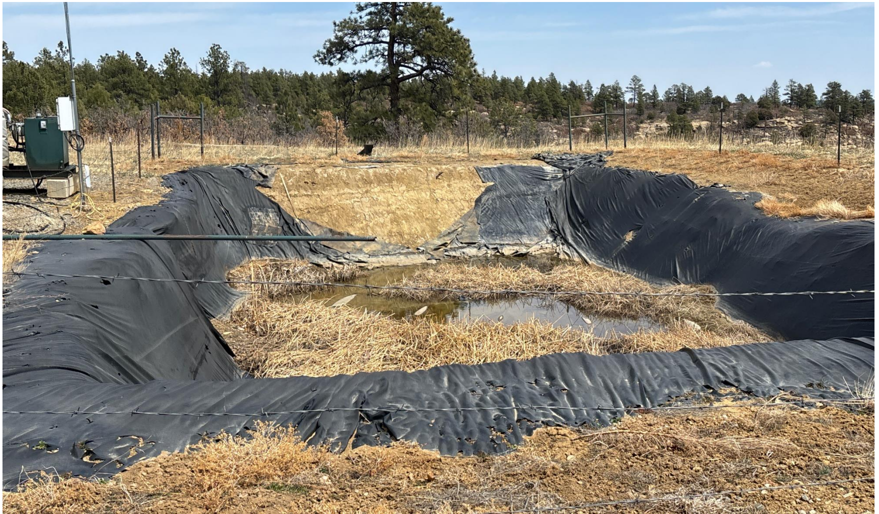
PHOTO 4: pit liner compromised (Rule 910). Reduce fluid level in pit, contact ECMC EPS staff for directives. CA DATE 4/9/2025
