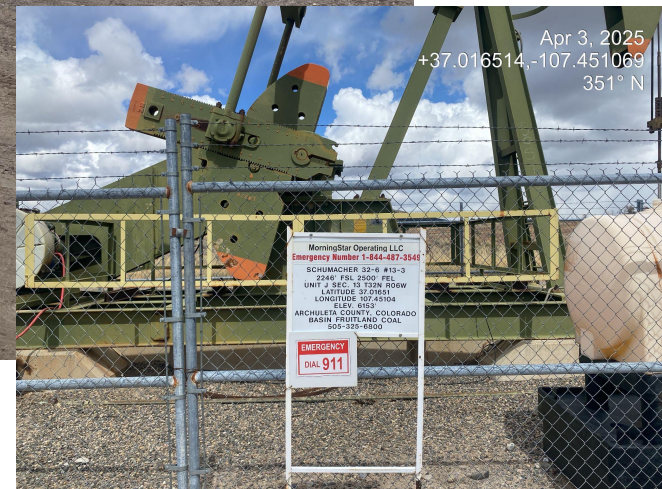
Photo 1. View of well pad taken from the access point facing center. Note: well sign missing API #.
