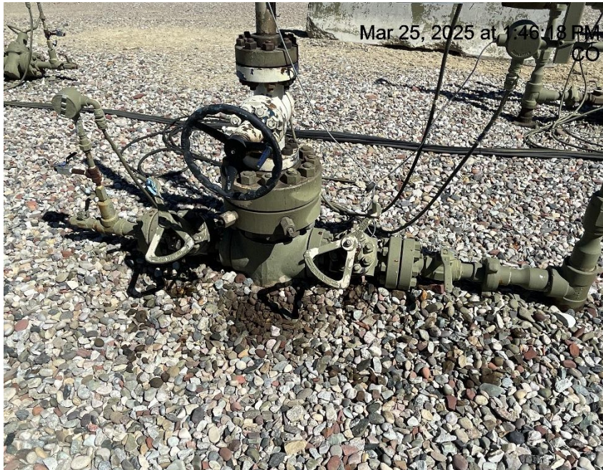
Photo # 7346 Staining near wellhead
