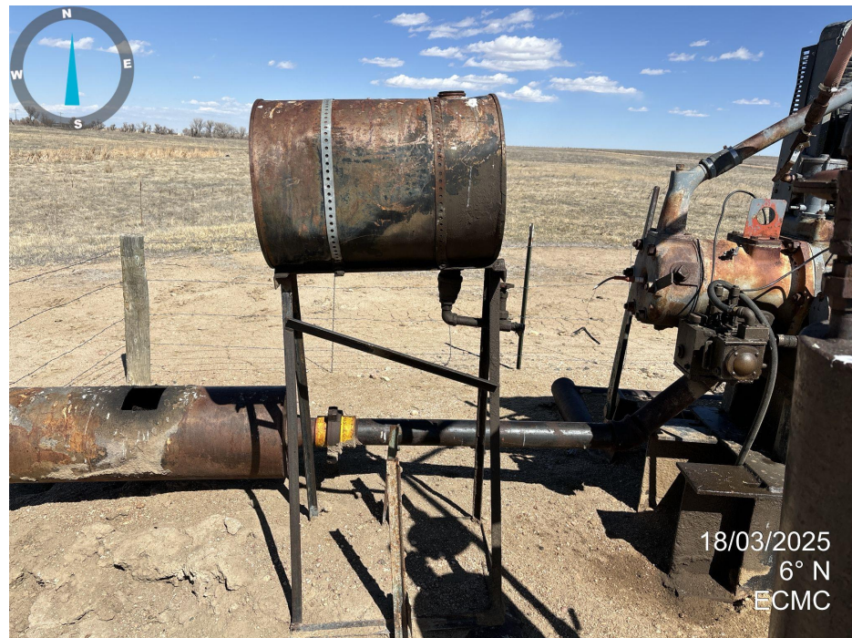
Photo 4. Barrel with no secondary containment.
