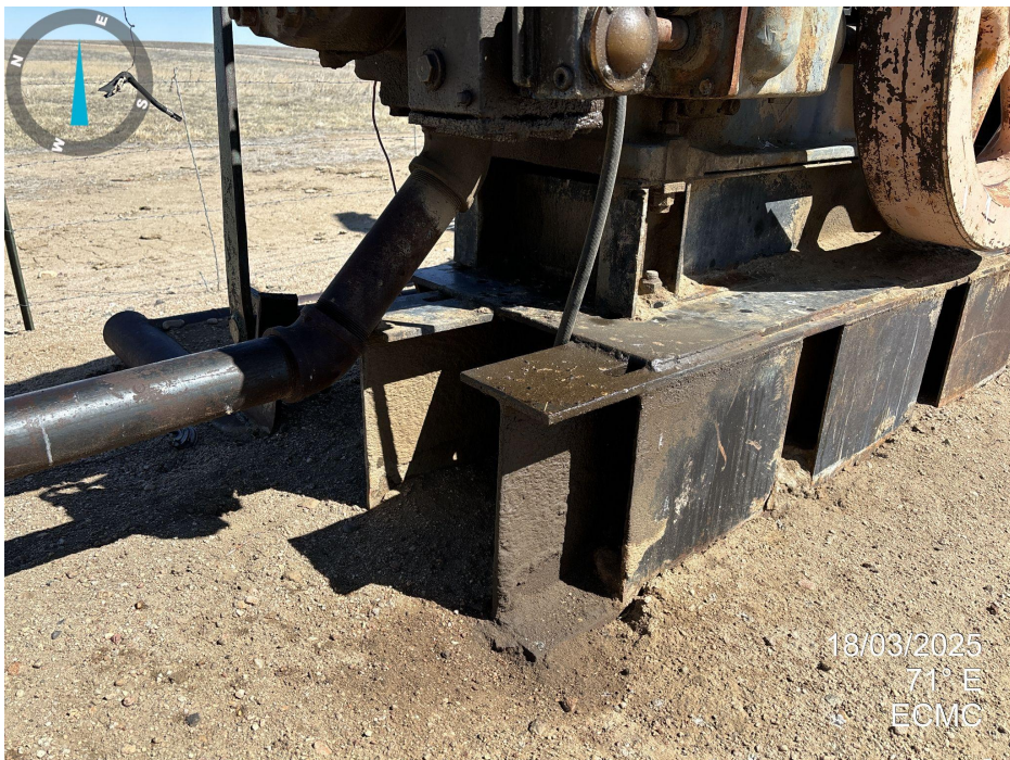
Photo 5. Stained soil beneath pumpjack motor.
