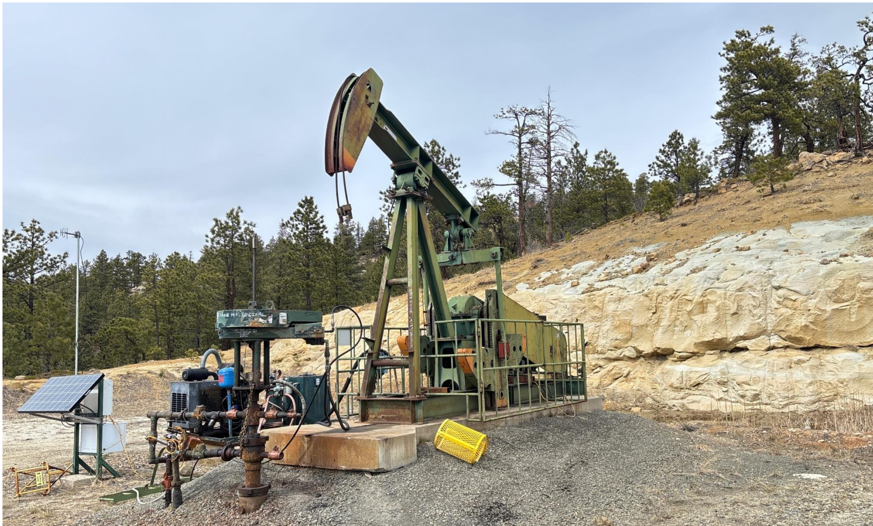
PHOTO 3: WELLHEAD AND EQUIPMENT. UNUSED EQUIPMENT ( A PC PUMP HAS BEEN INSTALLED ON THE WELL AND THE PUMPJACK HAS BEEN LEFT ON LOCATION). REMOVE UNUSED EQUIPMENT PER RULE 606. CA DATE 4/20/2025.
