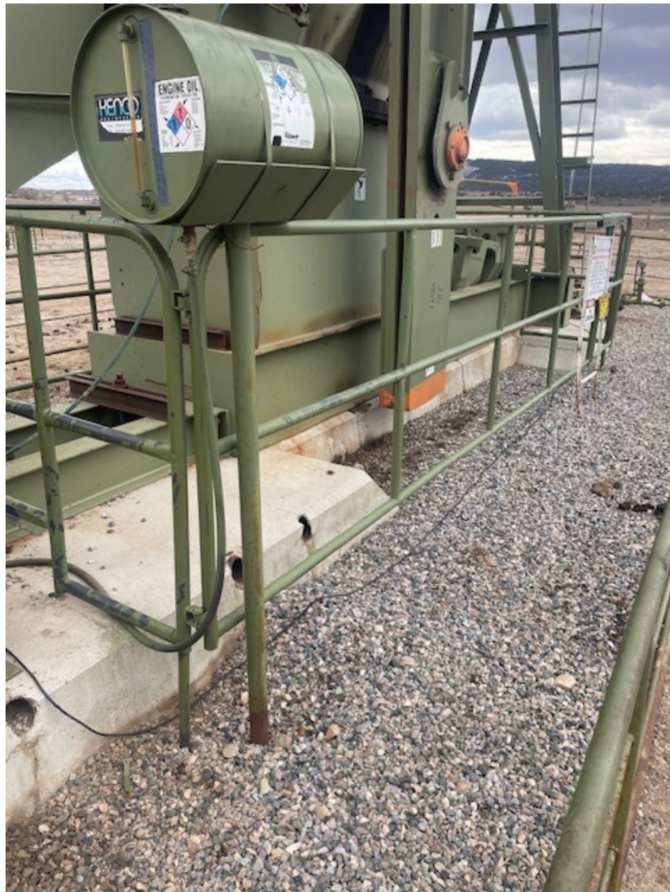
Containment was built around oil day tank.
