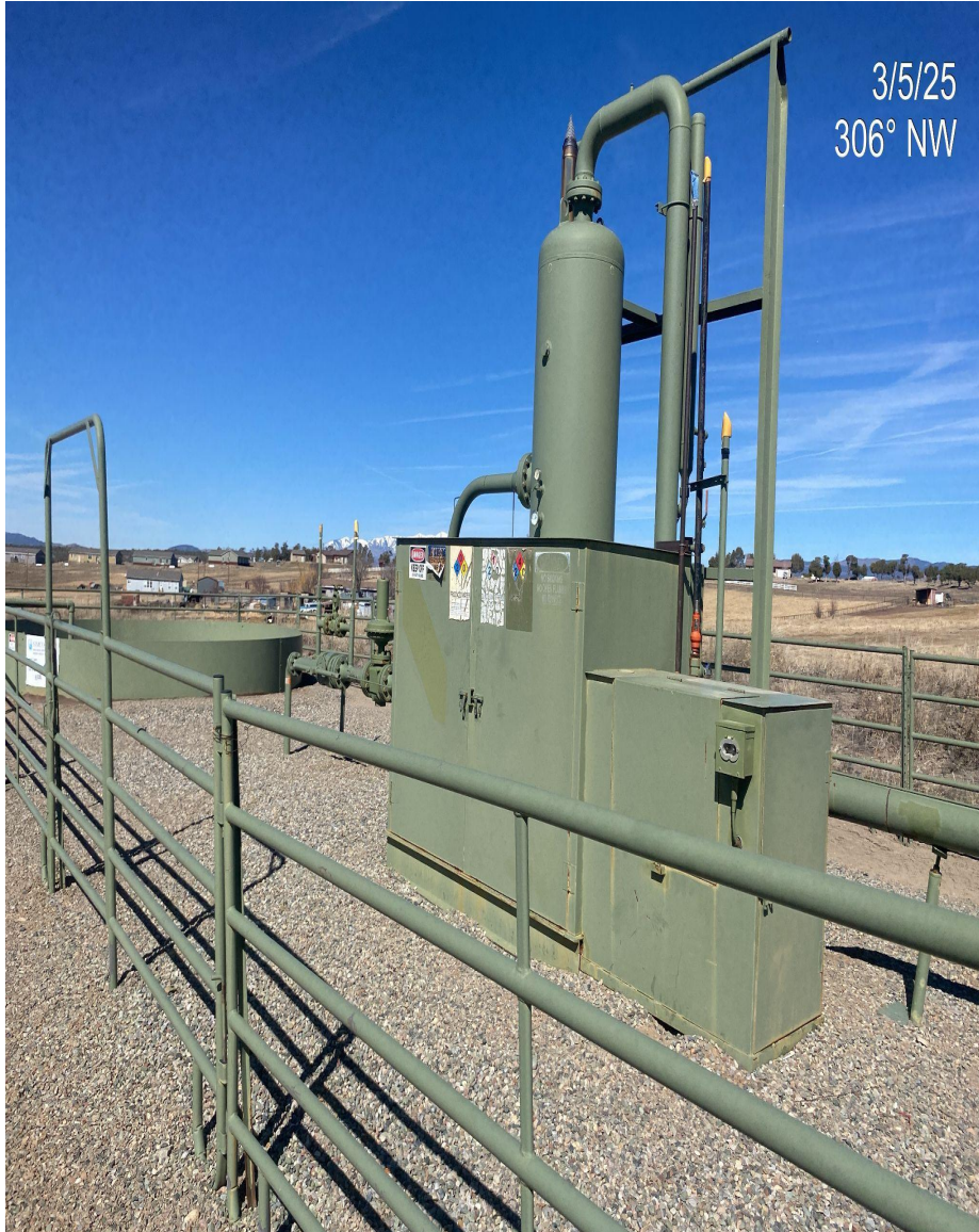
Photo 2. Labels at separator equipment have deteriorated and are no longer legible.
