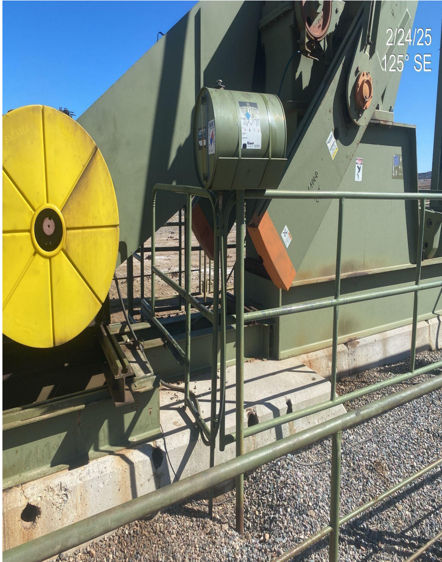
Photo 2. Spill prevention installed at oil tank is not sufficient.
