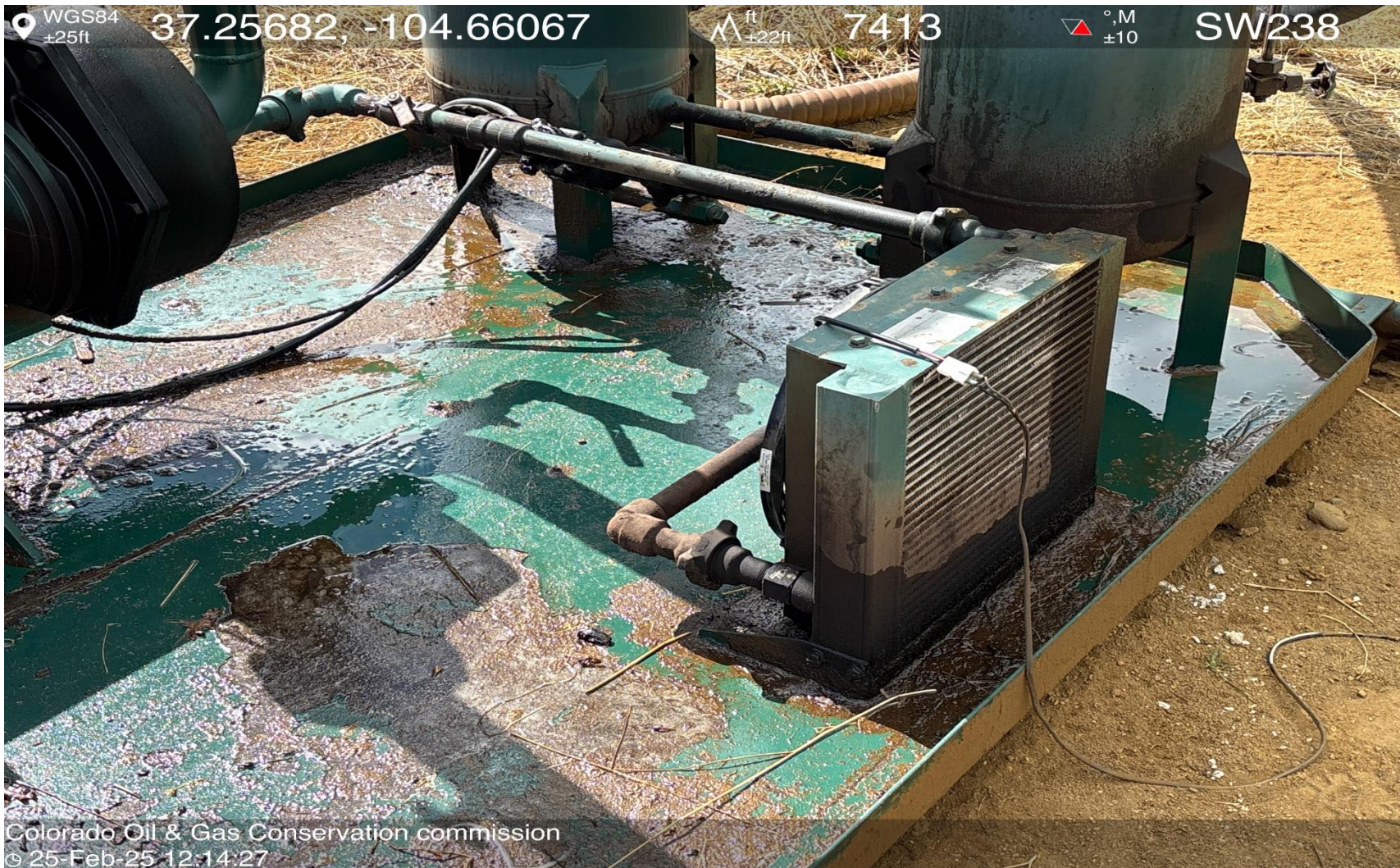
PHOTO 5: OILY WASTE IN COMPRESSOR SKID. DRAIN OILY WASTE REPAIR ALL LEAKS AND REMOVE OR TREAT IMPACTED SOIL PER RULE 1002..(2).D & 1002.f.(2)B, Comply with general provisions of the oil and gas act for wildlife protection AND SB-181. CA DATE 2-26-2025
