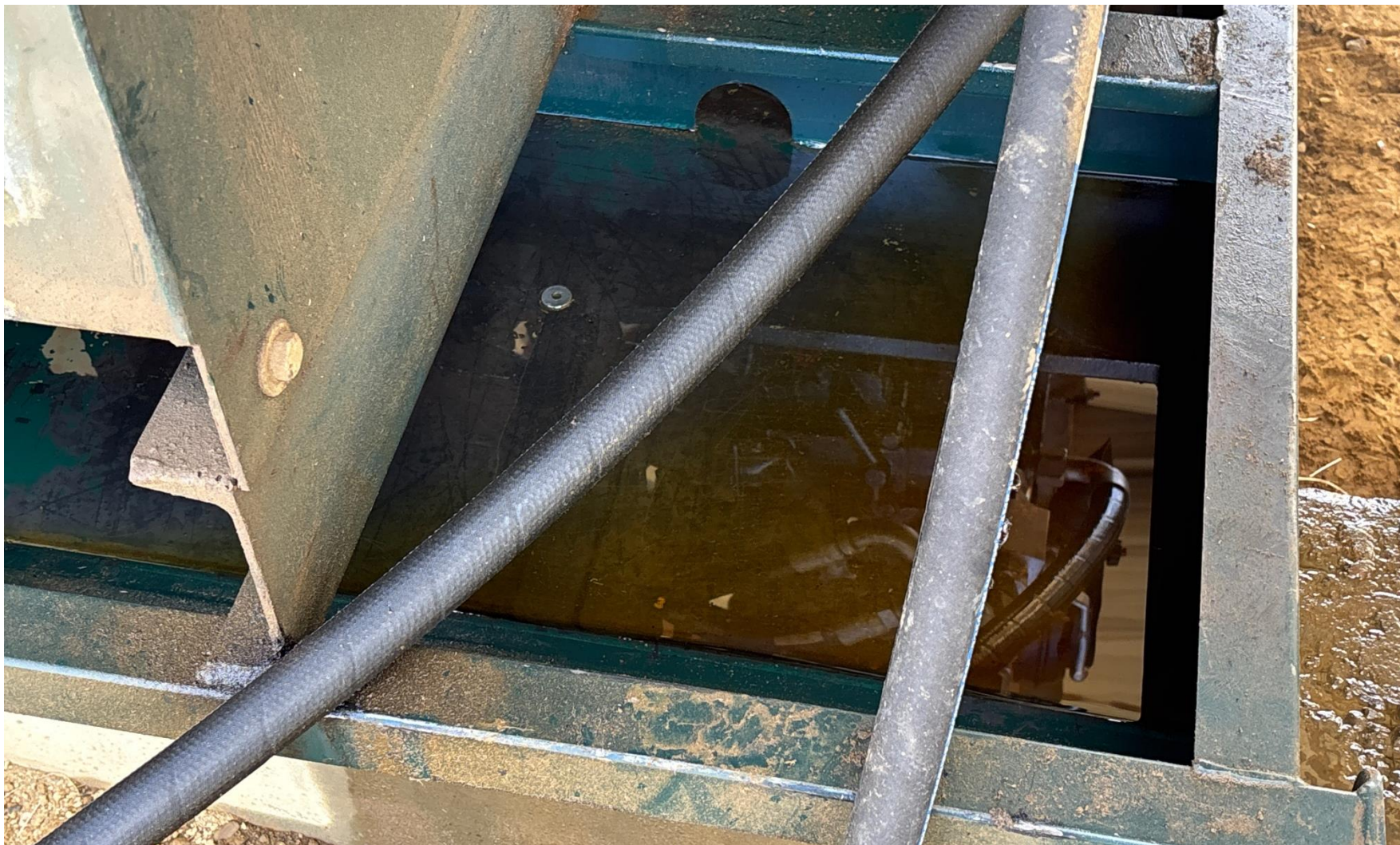
PHOTO 4: OILY WASTE IN PRIME MOVER ENGINE SKID. DRAIN OILY WASTE REPAIR ALL LEAKS AND REMOVE OR TREAT IMPACTED SOIL PER RULE 1002..(2).D & 1002.f.(2)B, Comply with general provisions of the oil and gas act for wildlife protection AND SB-181. CA DATE 2-26-2025
